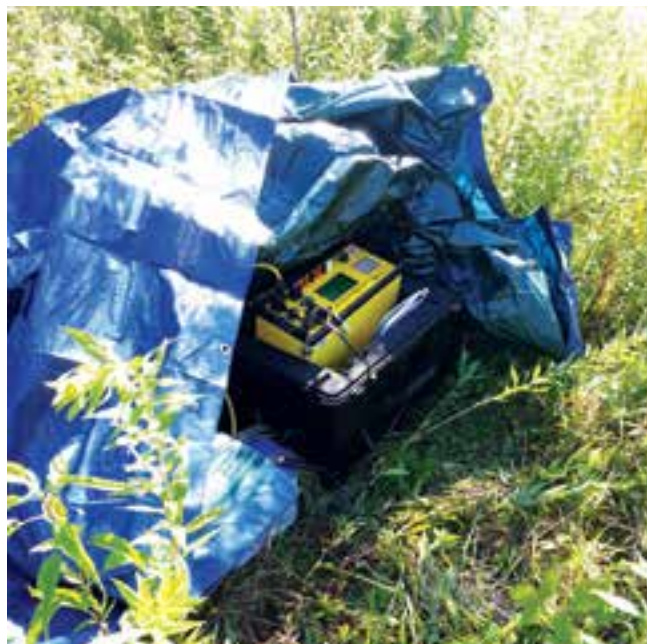
Figure 3. ERI equipment: AGI Earth Imager unit (above) and transect of electrodes connected by electrical cables (below). (PHOTO CREDIT: BREEYN GREER).
