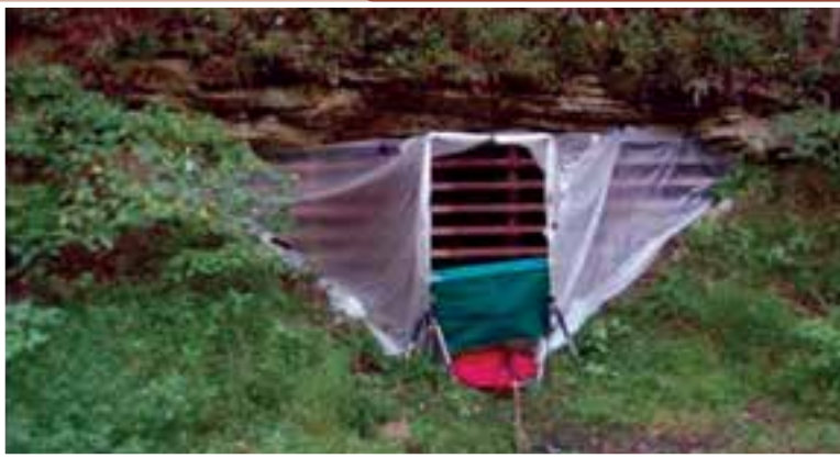
Figure 5. Standard bat gate with harp trap setup (PHOTO: SANDERS ENVIRONMENTAL).
