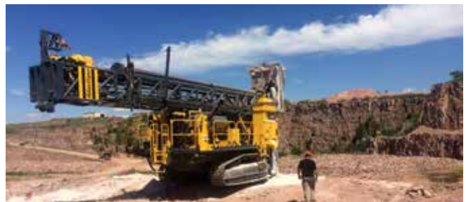
FIGURE 2 (Above and below). At Spencer Quarries students learned about mining Sioux Quartzite and got hands-on experience with the Pit Viper 351 – Blast Hole Drill made by Atlas Copco out of Wisconsin.
