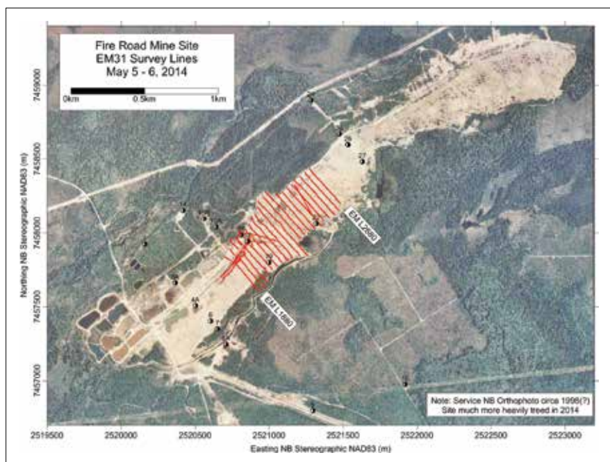
Figure 3. Layout of EM survey lines acquired on Fire Road Mine in early May 2014. Twenty-one EM31 survey lines were laid out at 40-m spacing with additional cross-lines in areas of special interest.
