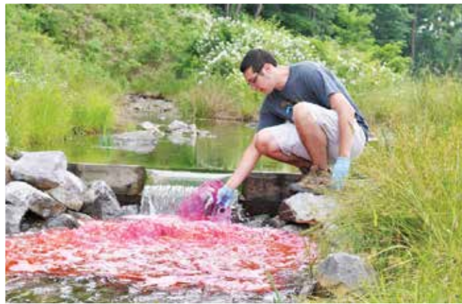
Figure 3. Rhodamine dye being added to the channel at the top weir to begin a tracer test to accurately determine residence time.
