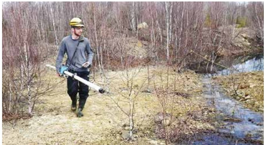
Figure 4. EM31 apparent conductivity surveying, May 2014. EM31 readings were integrated with positioning data from a differential GPS mounted on hard hat. Data were displayed and stored on a hand held data logger. (Photo KE Butler)
