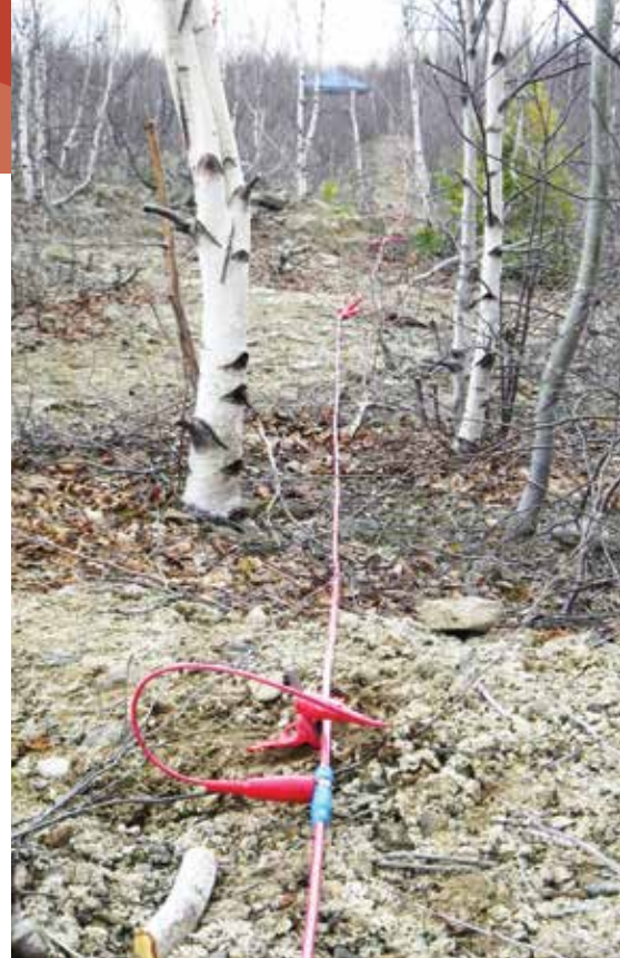
Figure 7. ERI survey line showing multi-conductor cable connected to 40 cm long stainless steel electrodes driven into the ground at 5 m intervals. (Photo KE Butler)
