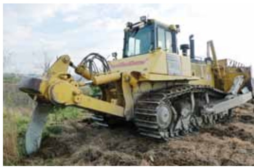
A bulldozer sinks a four-foot ripping shank into reclaimed mine soil in Pike County, KY.
