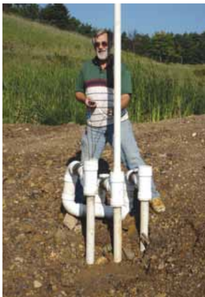
Figure 1. Bruce Leavitt measuring air velocity using an anemometer.
