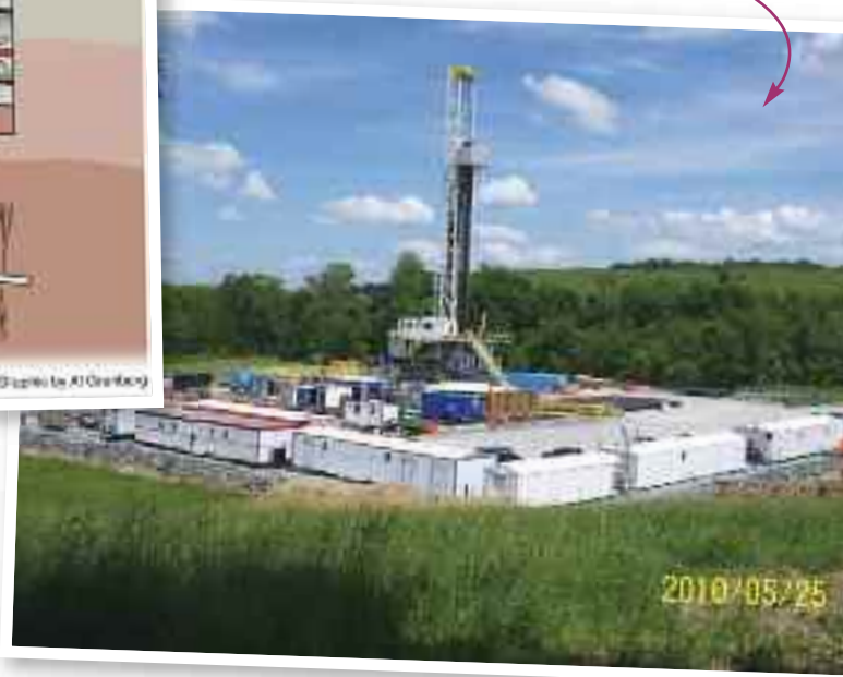
Figure 4. A Marcellus drill rig which is used to bore a vertical and horizontal well
