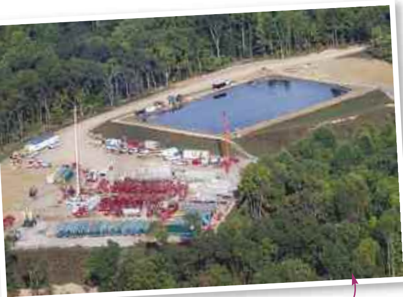
Figure 5. Marcellus Shale drilling site with water-holding structures and support facilities during drilling operations.
