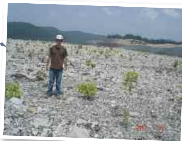
Figure 5. Unweathered gray sandstone in West Virginia originally dumped in piles and graded with one pass shows some weathering into smaller particles after two years, but has shown generally poor tree growth and poor colonization by native plants compared to weathered brown sandstone soil materials. The pH of these mine soils is >8.
