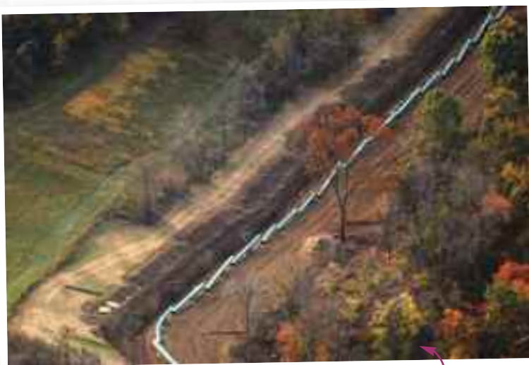
Figure 8. Pipelines are necessary for Marcellus Shale wells, and land disturbed for these pipeline corridors must be reclaimed.
