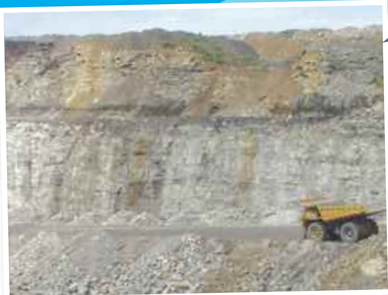
Figure 8. Weathered brown sandstone can be found immediately below the soil and it will often extend to about 30 feet from the surface. Under the brown sandstone material will be found the unweathered gray sandstone. The brown sandstone has been found to be a better material to place on the surface for forestry post-mining land uses.
