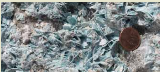
Picture 2: Kyanite crystals (blue) with quartzite and fine grained pyrite.. Kyanite is used in refractory bricks and on space shuttle heat shields.
