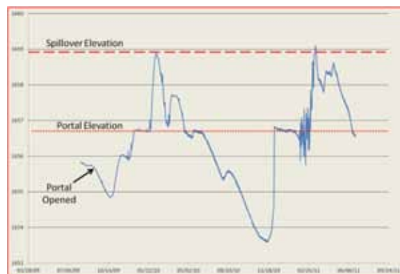
Figure 8. Shawmut Mine pool hydrograph
