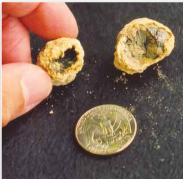
Figure 3 – Radial structure in partially decomposed pyrite nodules
