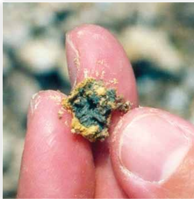
Figure 4 – Lack of coherence in decomposing pyrite nodule
