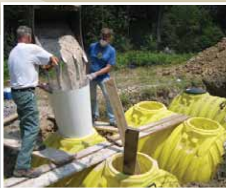
Figure 5. President of the Clearfield Creek Watershed Association, Earl Smithmeyer, and Penn State undergraduate Honors student, Sara Goots, add a mixture of crab shells and spent mushroom compost into one of the pilot reactors.
