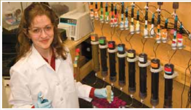
Figure 3. Dr. Brennan and the continuous-flow column system that her research group uses to test different substrate combinations for the treatment of high-strength acid mine drainage. PHOTO CREDIT: SARA BRENNEN.
