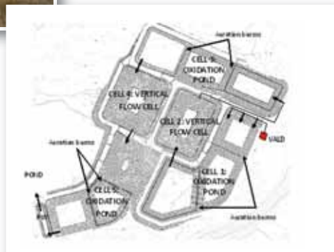
Below: Figure 1. Schematic of Rock Island #7 passive treatment system with discharge point shown in red. (BASE DRAWING COURTESY OF BURNS AND MCDONNELL, 2004)
