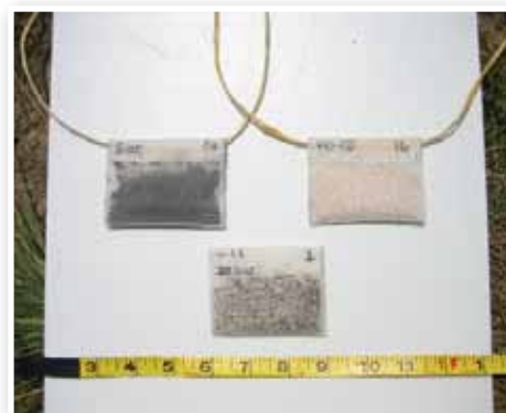
Figure 8. Permeable substrate bags inserted into the pilot reactors for later microbial community analysis, arranged left to right: spent mushroom compost and limestone chips, crab shell and spent mushroom compost, and crab shell only.
