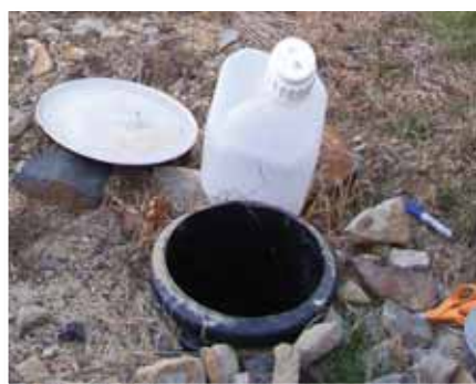
Figure 2. Pan lysimeter installation in the center of a plot (top). The leveled pan in the foreground drained to a carboy at the bottom of the PVC well in the background. The pan was then covered with the original soil removed from the trench. Plastic carboys were placed in each well to collect the leachate (bottom).
