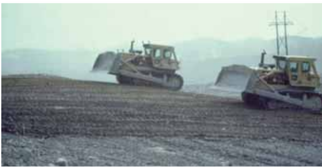
Photo 4. Soil compaction due to equipment operation on mine soils hinders survival and growth of planted trees. "Tracking in" operations, such as those shown in the photo, are NOT recommended for mine sites on which trees will be planted, unless required to stabilize steep slopes.
