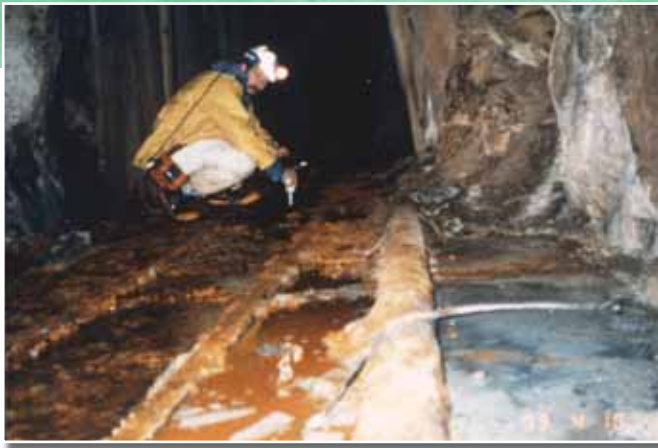
Figure 6. – Author Testing Iron and Zinc Bearing MIW at an Abandoned Pb-Zn Mine in Colorado
