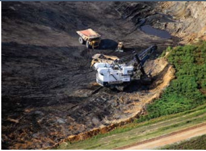
Figure 2. Truck and shovel operation salvaging red oxidized overburden as a suitable substitute topsoil material.
