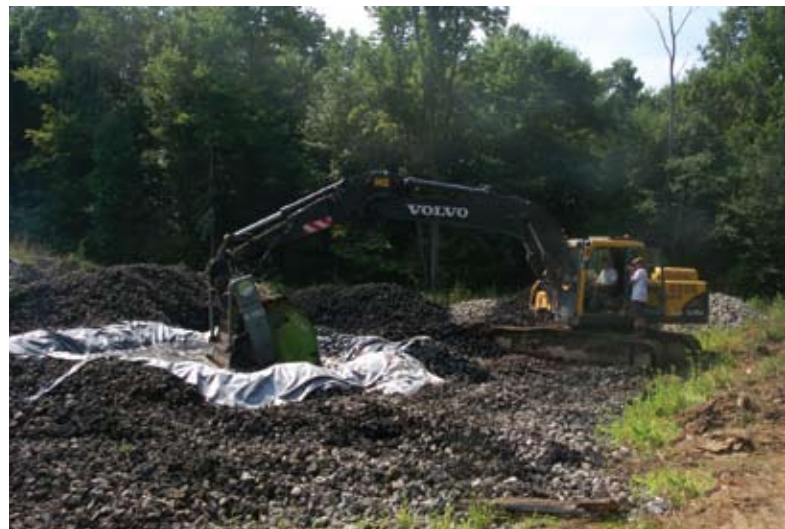
Figure 2. Excavator with FlipScreen attachment “washing” manganese covered limestone.
