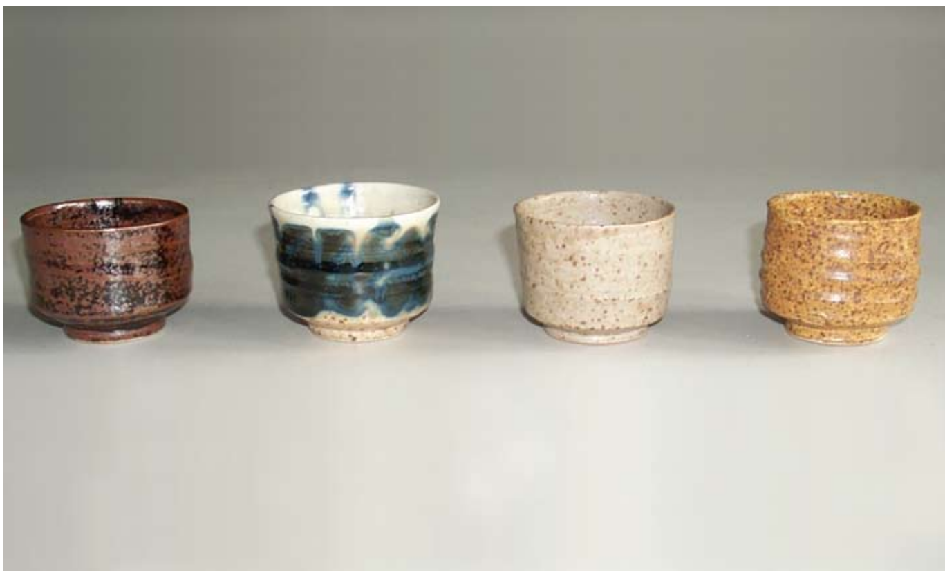
Figure 5: Examples of pottery with glazes using recovered manganese material and iron oxides formed at low pH.
