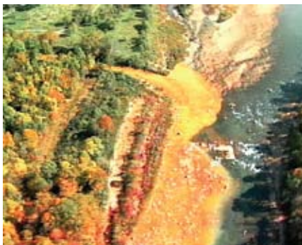
Figure 2. Acid mine drainage from an underground mine blowout spilled into Muddy Creek, which flowed into the Cheat River.
