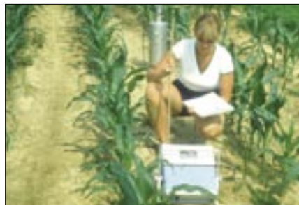
Photo 6. Bulk density data using a gamma density probe.
