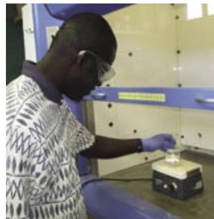
Fig. 13: Acid Base Accounting test
