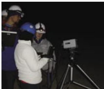
Fig. 9: Measuring the temperature of rock pile surface with a thermal camera at about 2 a.m.
