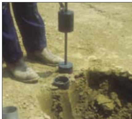
Photo 5. Initial bulk density sampling, cores.
