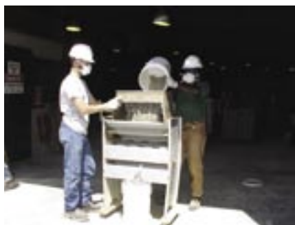
Fig. 2: Splitting drill cuttings with a soil splitter
