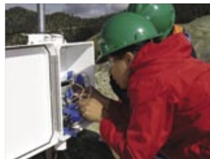
Fig. 5: Connecting tensiometers to a data logger powered by solar cells
