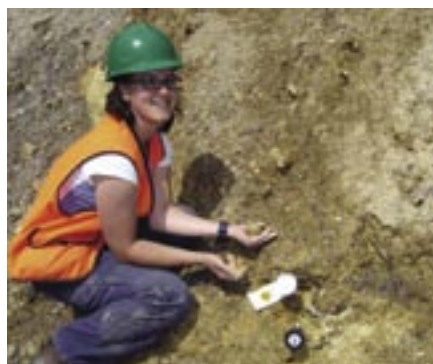
Fig. 8: Measuring soil temperature, pH and degree of saturation
