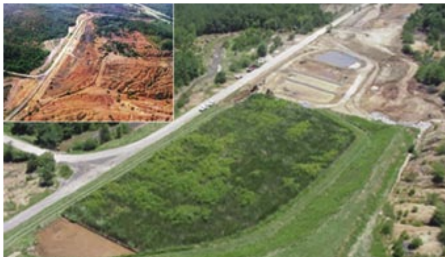
Picture 7: The McPherson roast yard is now a passive treatment system. In addition to neutralizing the stream, the wetland liner prevents infiltration of mine wastes beneath.
