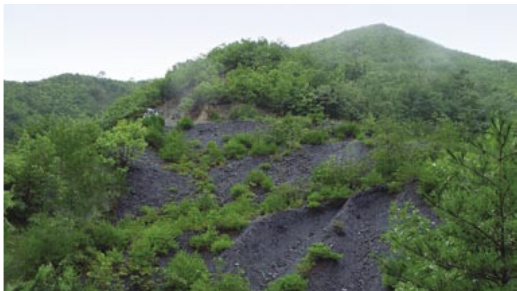
Picture 2: Large waste coal piles (gob) are found throughout the eastern coal mining area in South Korea. Runoff from this materials is acid mine drainage.
