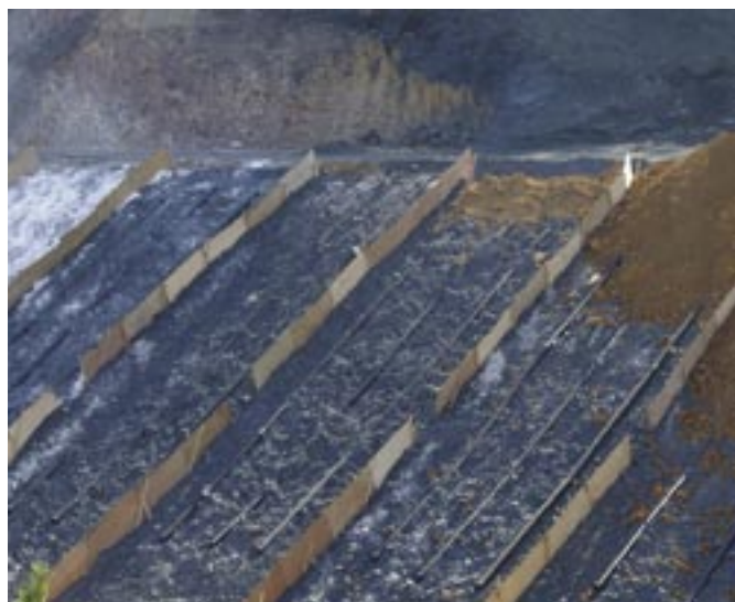
Picture 3: Plots were 20 m long by 5 m wide on a 56% slope. Plot 1 with coal waste only can be seen in the upper left hand corner with calcite, lime cake, and topsoil treatments extending to the right (see Table 1). Pipes were installed to collect the drainage.
