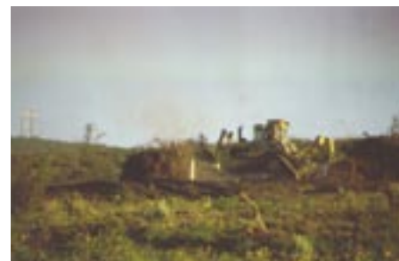
Picture 6: Materials such as topsoil and rocks are collected before mining for placement in drainage channels on adjacent reclaimed lands.
