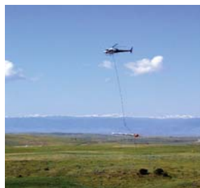
Figure 2. Helicopter electromagnetic survey of coalbed methane field in the Powder River Basin in Wyoming
