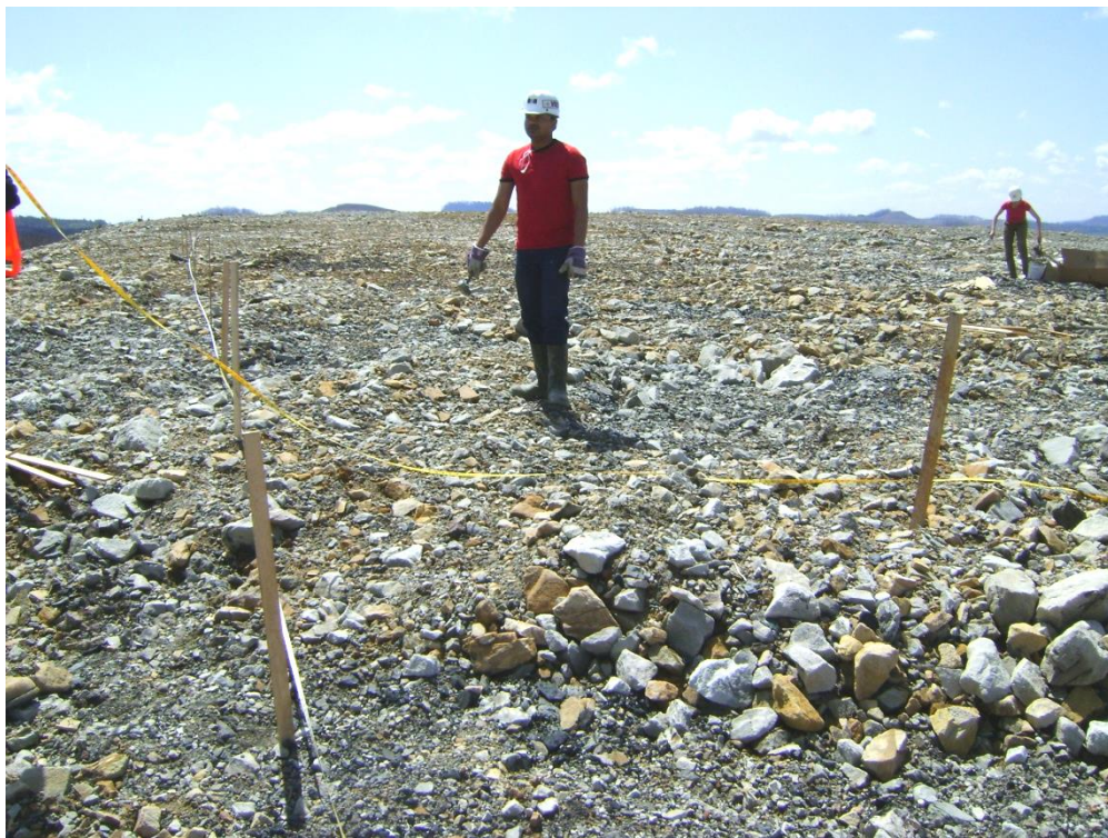
Figure 4. The 0.3-ha experimental area of gray sandstone at Nicholas was constructed in 2009 with primarily gray sandstone and some brown material, and graded by bulldozers.
