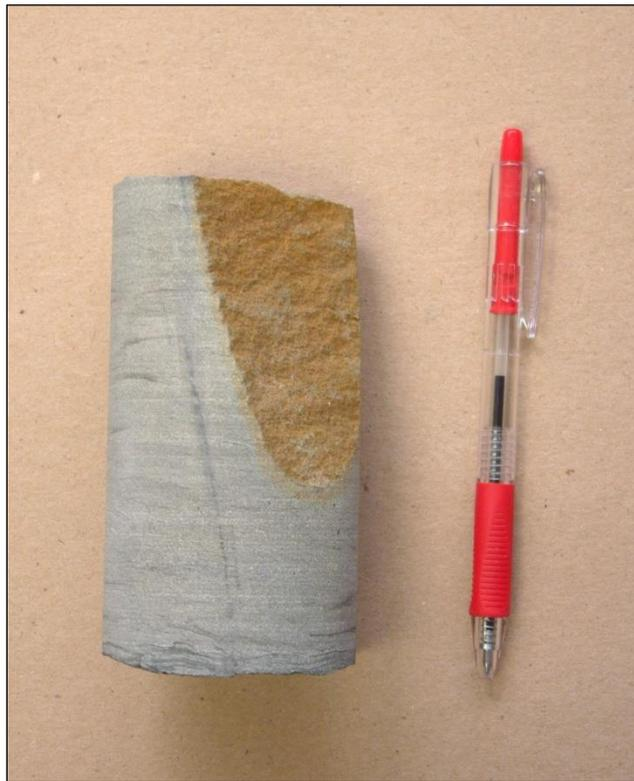
Figure 14. Interburden core sample exhibiting high angle subsidence-induced fracture with iron staining due to ground water contact in a siltstone unit.
