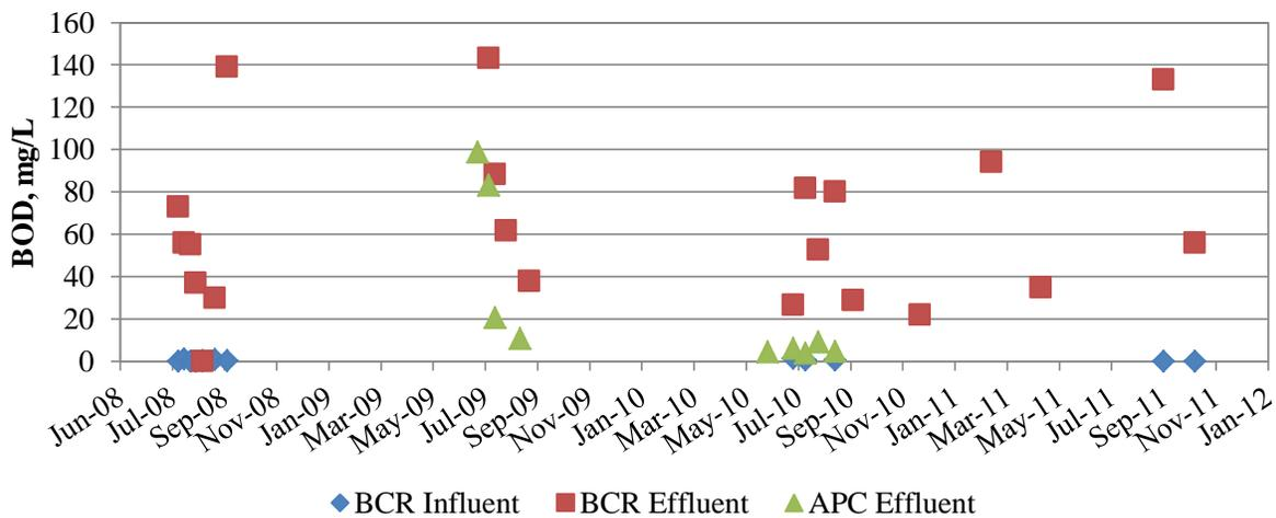
Figure 10. BOD in BCR Influent, BCR Effluent, and APC Effluent
