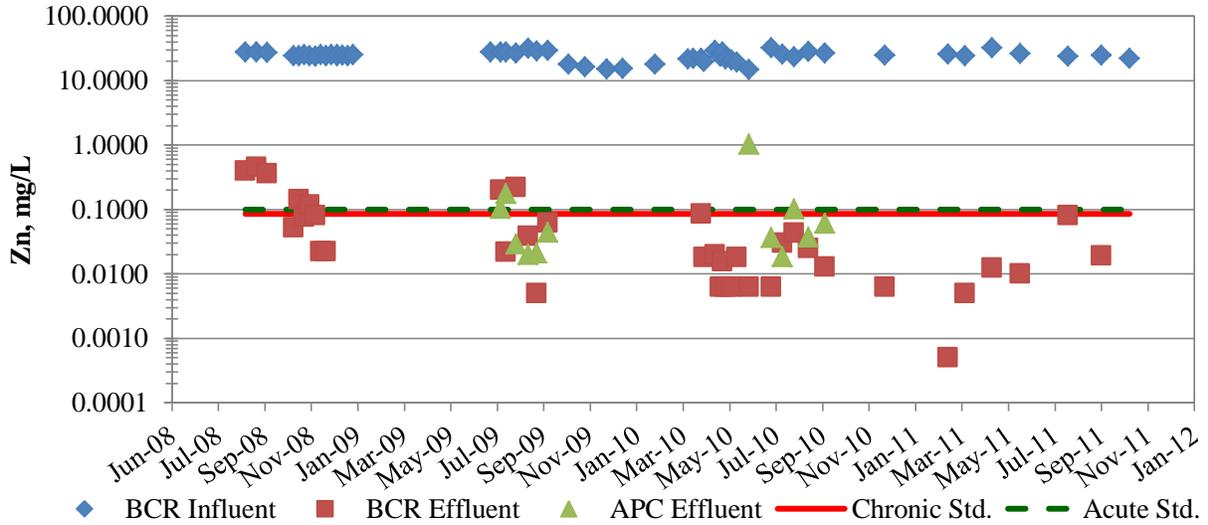
Figure 8. Dissolved Zn in BCR Influent, BCR, Effluent, and APC Effluent
