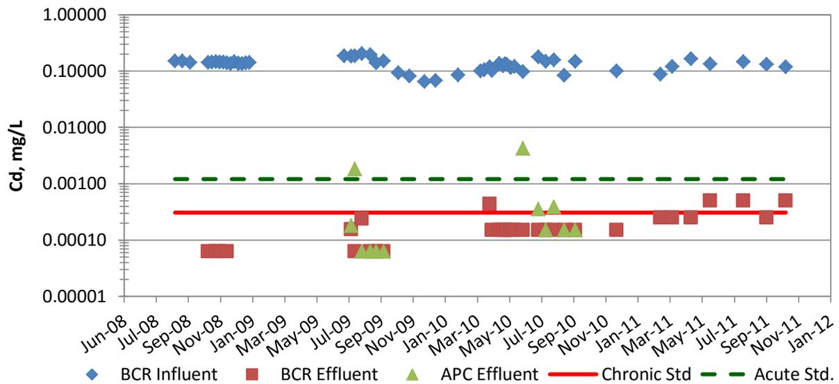
Figure 3. Dissolved cadmium in BCR Influent, BCR, Effluent, and APC Effluent
