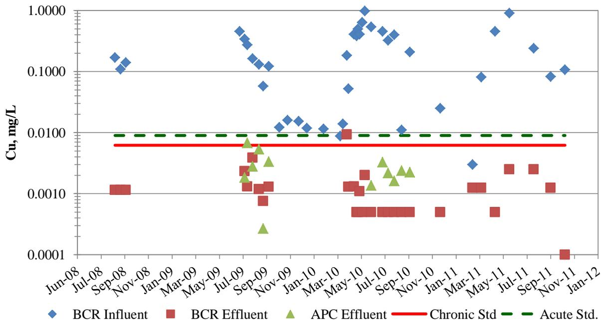
Figure 4. Dissolved copper in BCR Influent, BCR, Effluent, and APC Effluent
