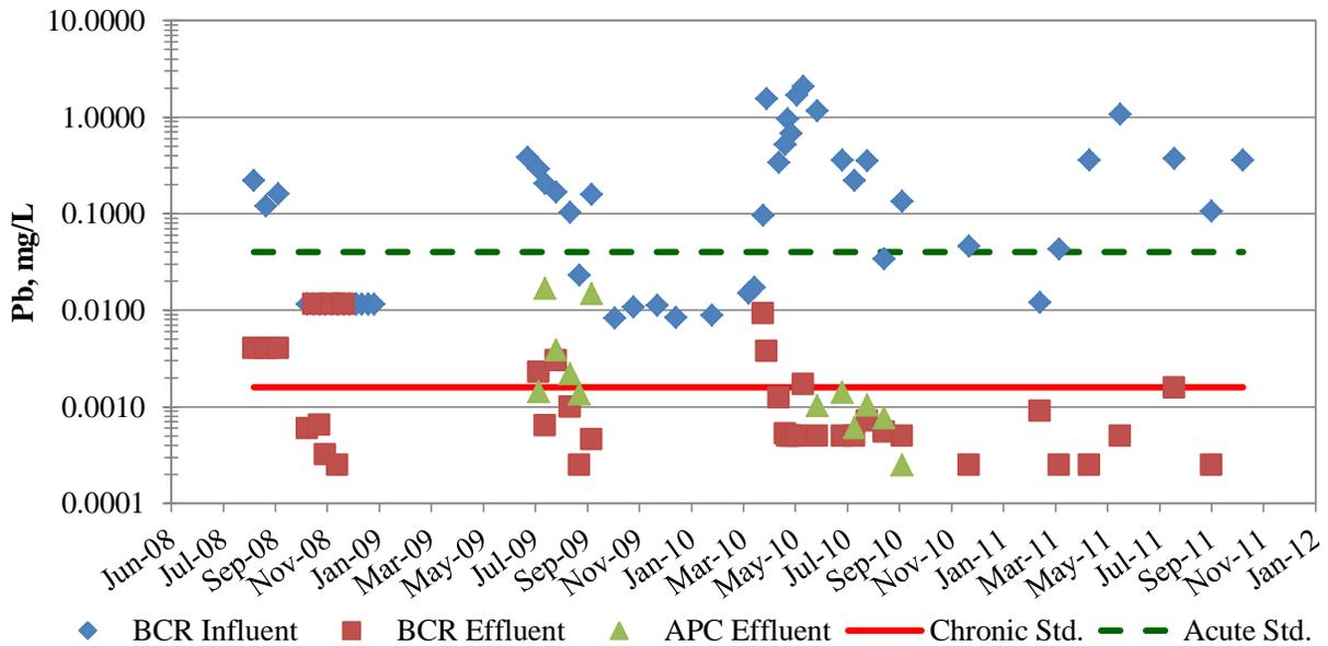
Figure 6. Dissolved Pb in BCR Influent, BCR, Effluent, and APC Effluent
