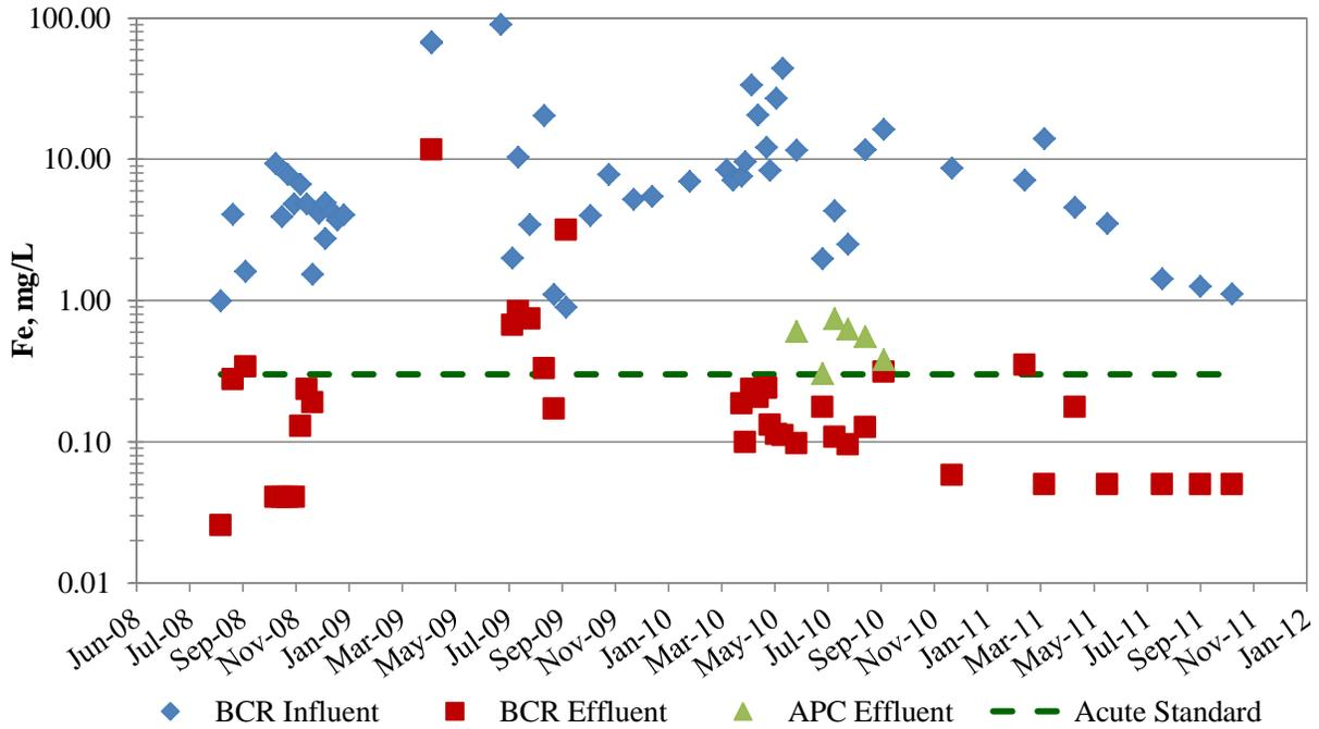
Figure 5. Total iron in BCR Influent, BCR Effluent, and APC Effluent
