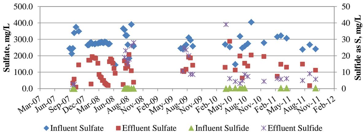
Figure 9. Sulfate and Sulfide in BCR Influent and BCR Effluent
