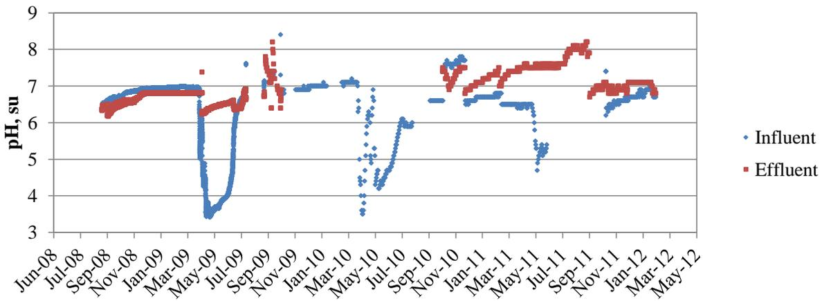
Figure 1. pH of BCR Influent and Effluent
