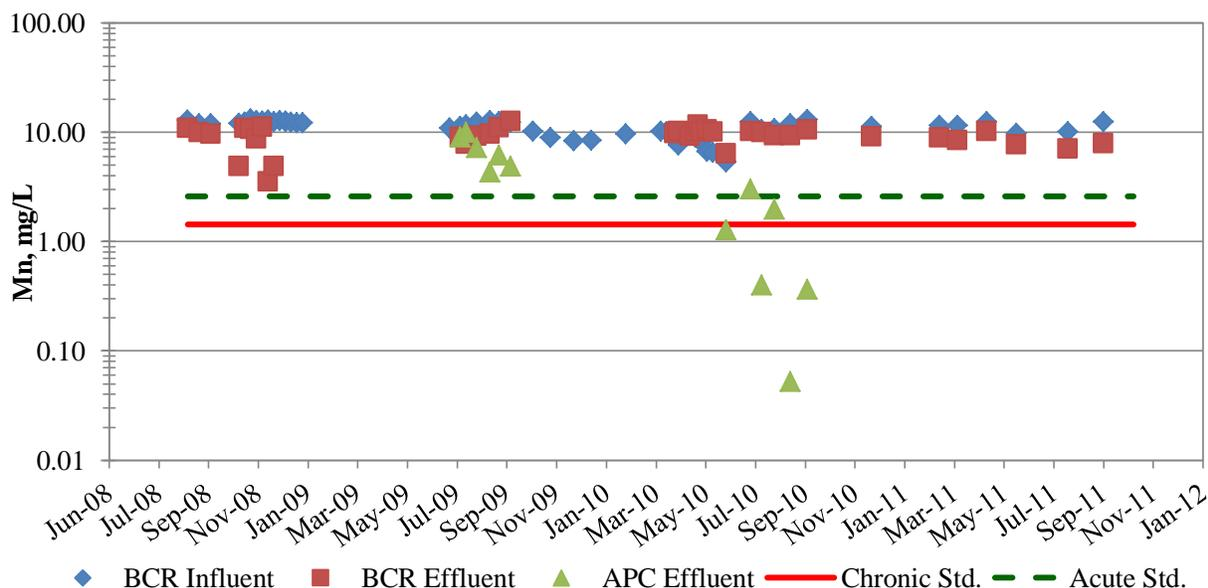
Figure 7. Dissolved manganese in BCR Influent, BCR, Effluent, and APC Effluent
