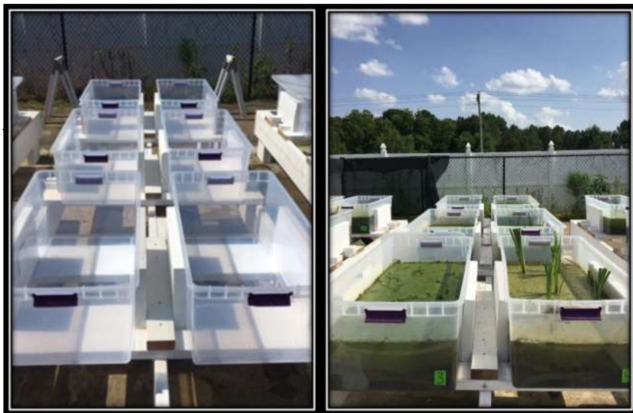
Figure 2. Constructed wetland microcosms made from 115-L plastic containers (left). Microcosms contained 0.035 m 3 of a Catalpa silty clay loam planted to five aquatic macrophytes, or unplanted, and flooded with 30 L of water at 0, 500, or 1000 ppb Se as selenite or selenate (right).
