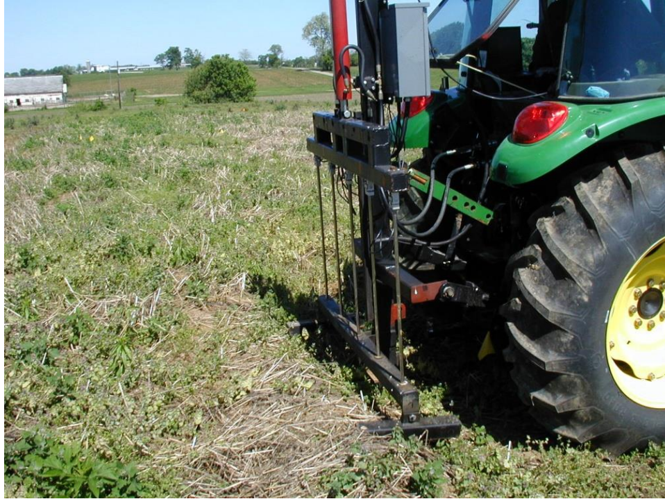
Figure 5. Five probe mechanical soil cone penetrometer system.
