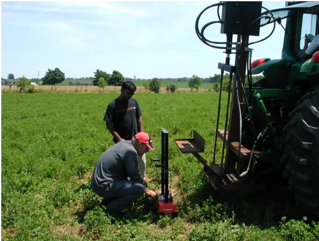
Figure 4. Dual probe soil moisture density gauge with tractor-mounted apparatus to create vertical access holes.
