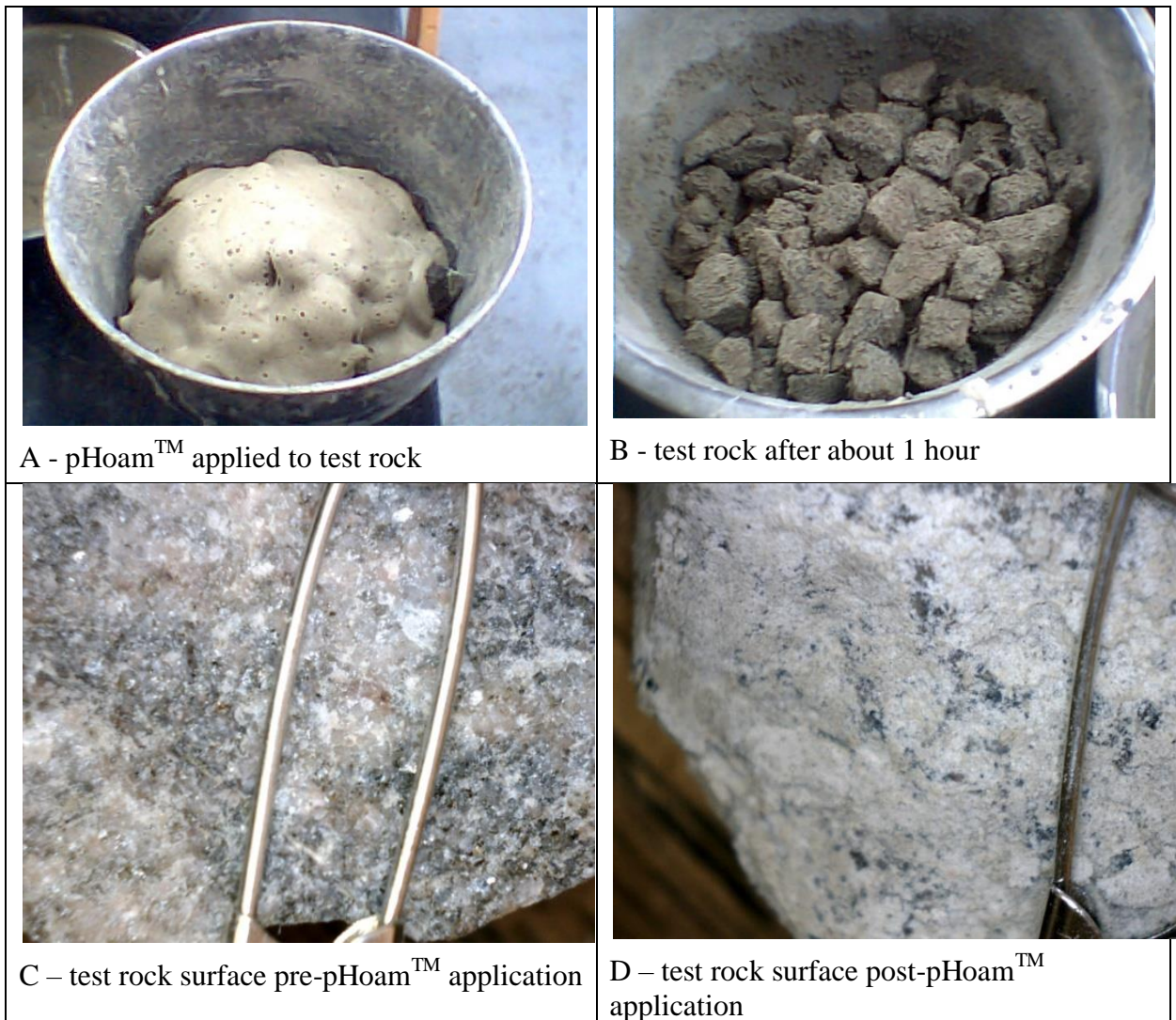
Figure 5. Laboratory application of pHoam™ to a clean gravel test rock
