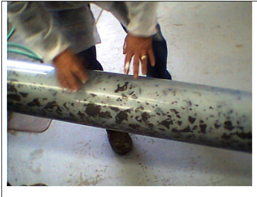
Figure 6. Gravel in column is encapsulated with pHoam™ after feed was suspended
