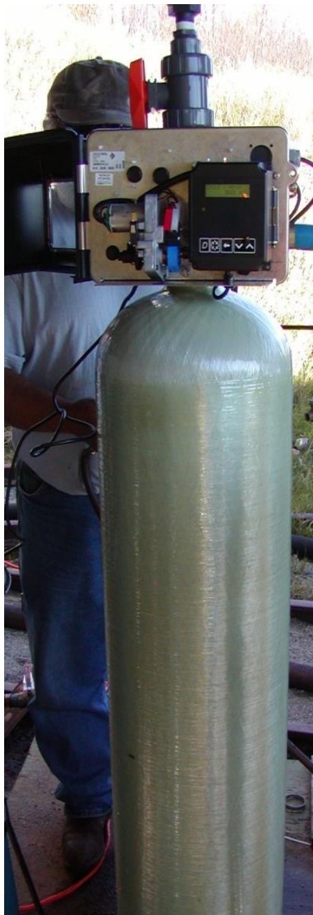
Figure 4. 105 liter fiberglass tank with control unit used in pilot test
