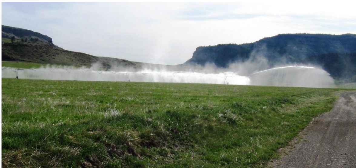
Figure 1. The off-site land application disposal (LAD) facility center pivot system. The center pivots are used to provide a polishing treatment for nitrate and dispose of excess mine waters. These center pivots use high pressure nozzles and “drops” that are oriented upward to evaporate as much water as possible, rather than deliver it to soil. This orientation evaporates an average of about 30 percent of the end-of-pipe water volume. An additional 85 to 90 percent removal of nitrate is achieved during polishing treatment by LAD (SMC 2006). DEQ photo.
