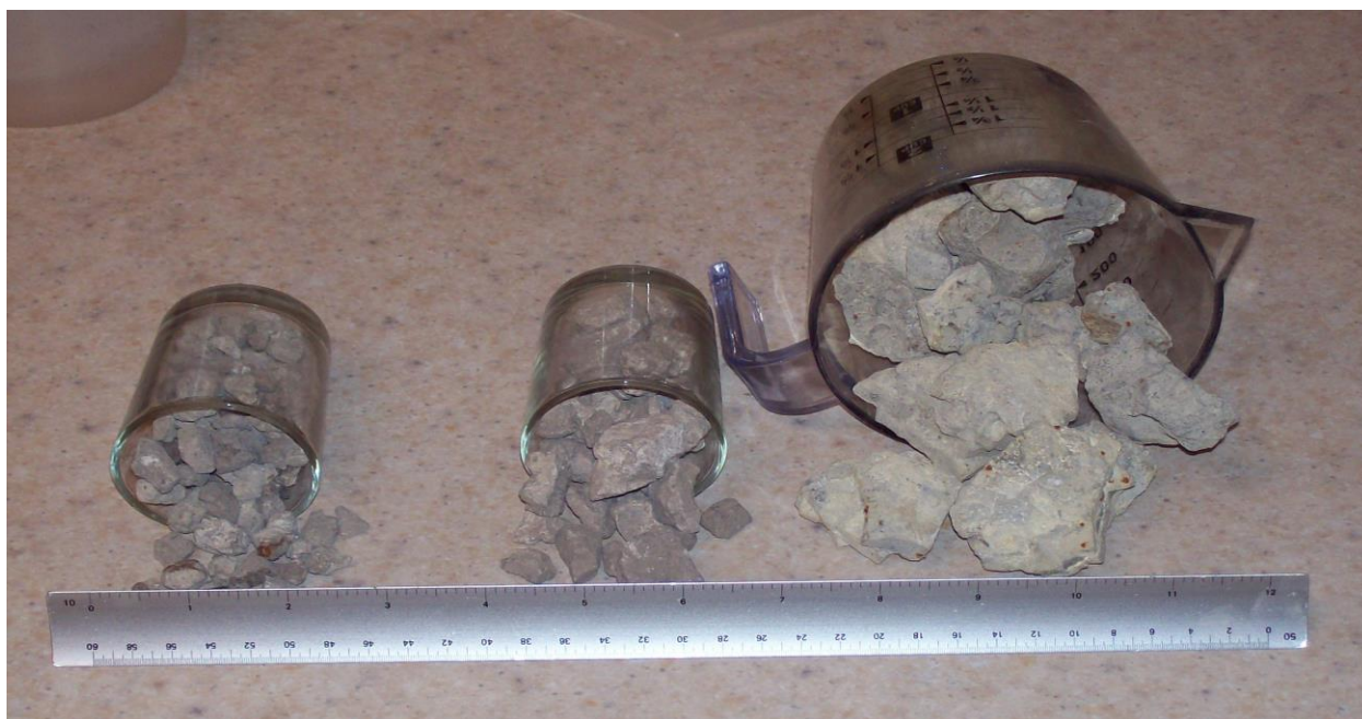
Figure 2. Three different sizes of Judy Hollow steel slag materials used in tests.
