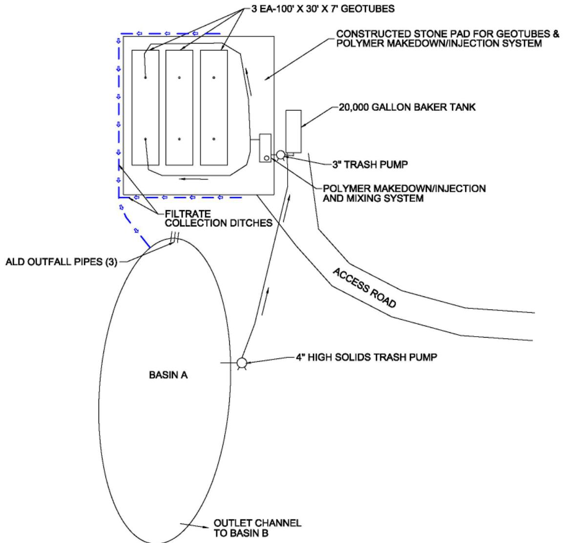
Figure 3. Sludge removal and dewatering system schematic.
