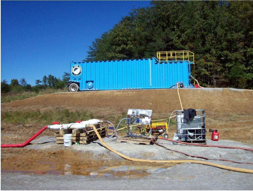
Figure 5. Photo of the polymer makedown system and 20,000 gallon stainless steel tank components of the sludge dewatering process at the RA1 site.
