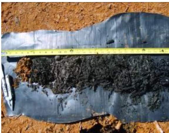
Figure 8. Disturbed substrate sample with top of substrate on the left.
