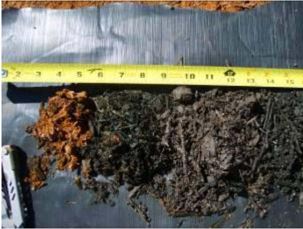
Figure 9. 0" – 14" depth showing iron hydroxide zone (0" – 1"), black sulfide zone (1" – 8") and aluminum zone (8" – 14")
