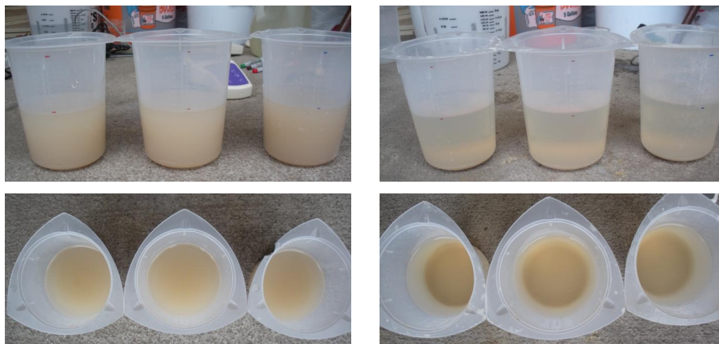
Figure 5 - Samples Immediately after Sample Collection and After 24 Hours of Settling
