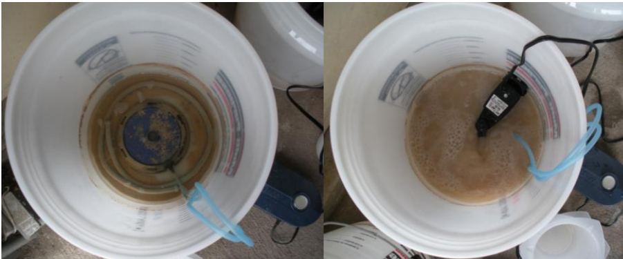
Figure 4 - Aerobic Lagoon Before and After Inserting Recirculating Pump for Solids Suspension
