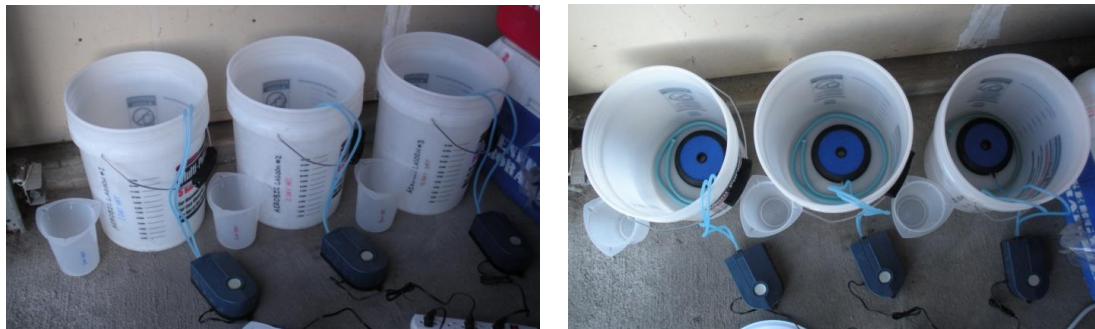
Figure 2 - Aerobic Lagoon Lab Test Experimental Setup
