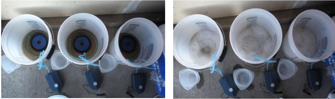
Figure 3 - Aerobic Lagoons Before and After Aeration (left to right: 1 day HRT, 2 day HRT, and 4 day HRT)
