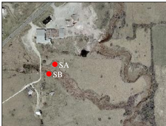
Figure 2. Aerial photograph of study site prior to passive treatment system construction showing location of mine drainage discharges SA and SB, receiving stream and proximity of local residential and commercial developments.
