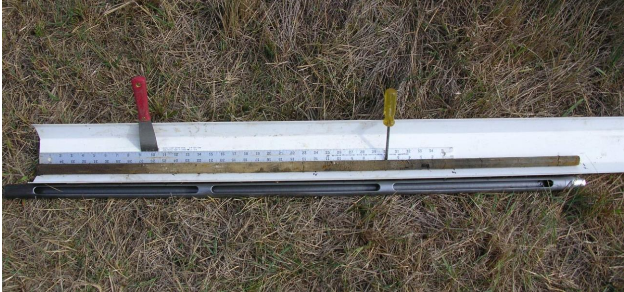
Figure 6. Soil core retrieved from a probe location for observation. Topsoil was present from 0 to 25.4 cm (10 in), subsoil was present from 25.4 cm (10 in) to 76.2 cm (30 in), and spoil was present below the subsoil.
