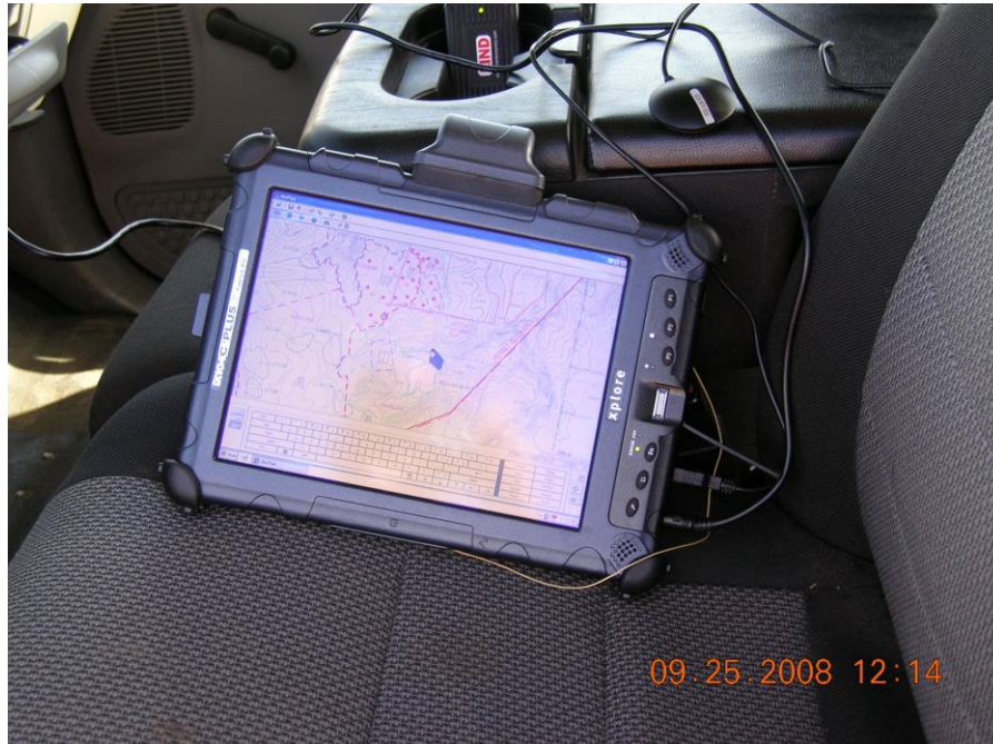
Figure 3. Xplore Technologies tablet computer used in collecting the attributes of soil probe locations
