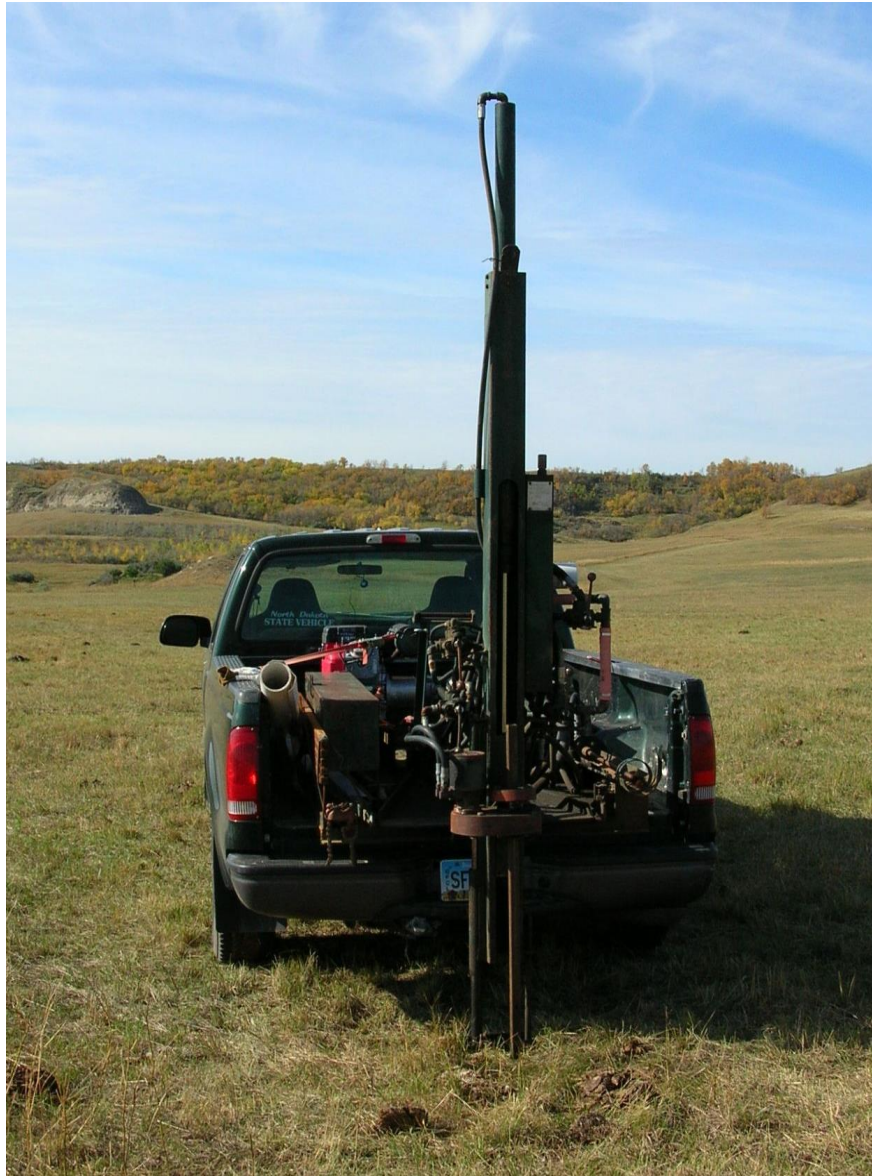
Figure 5. Truck mounted Giddings Machine Company soil probe used to collect soil cores for thickness observations.
