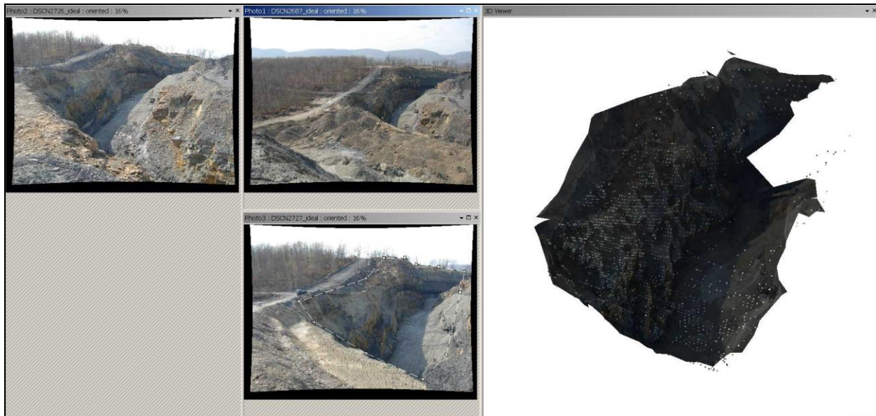
Figure 3 Point cloud and triangulated mesh created by DSM.
