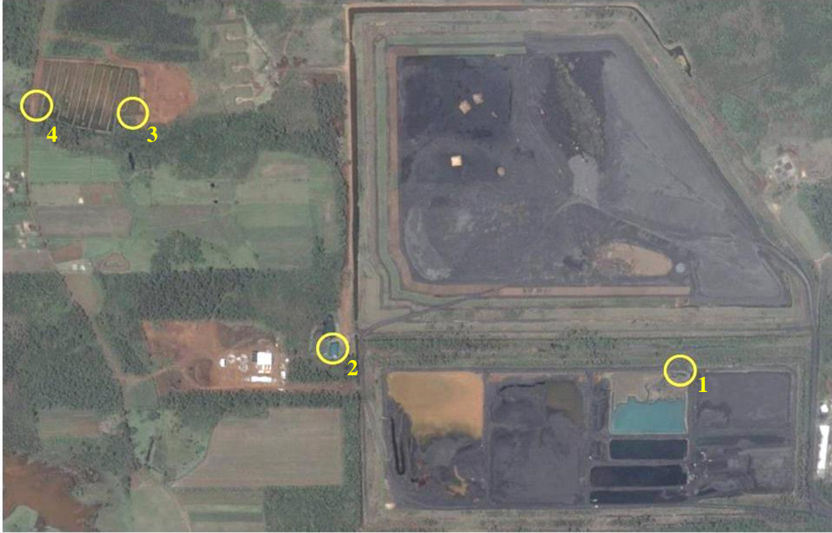
Figure 2. Locations of sample collection stations 1 (pH control and precipitation), 2 (second damping pond outlet), 3 (wetland inlet), and 4 (wetland outlet), marked with yellow circles. (Source: Image base captured from Google Earth).
