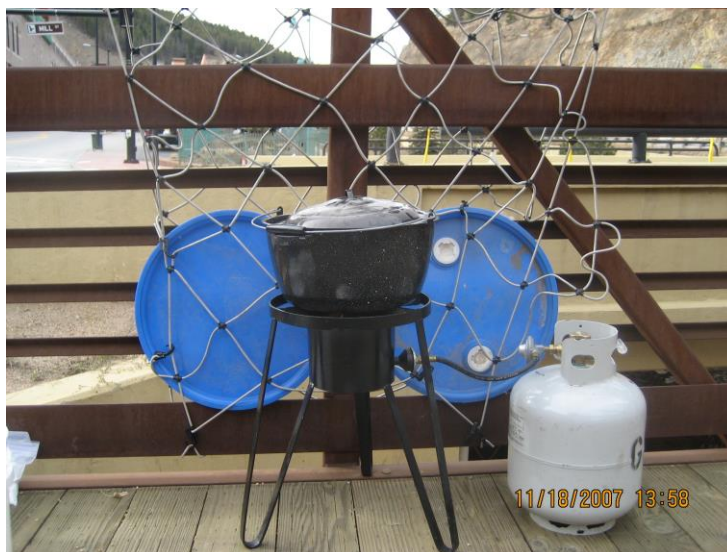
Figure 4. On-site heating of MIW prior to CBD addition on November 18, 2007.
