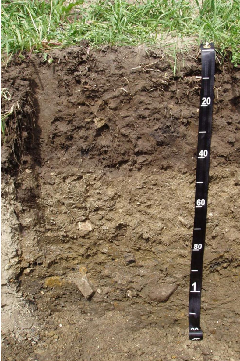
Figure 6. Profile of a reclaimed soil after surface mining for coal (note reduced porosity below 70 cm).
