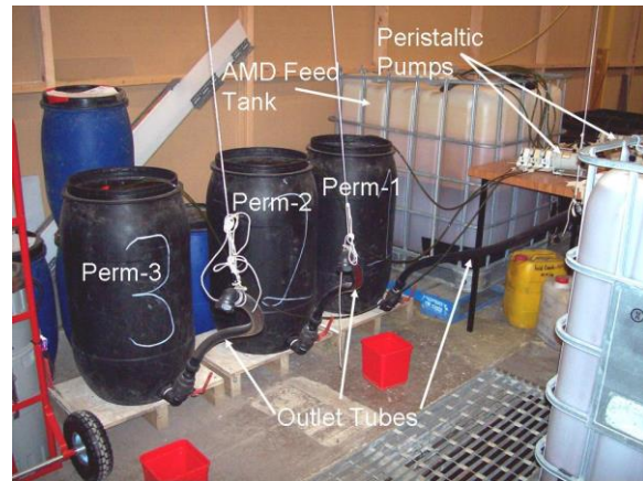
Figure 7. Mesocosm SRBRs (Perm-1, Perm-2 and Perm-3) and AMD feed tank.
