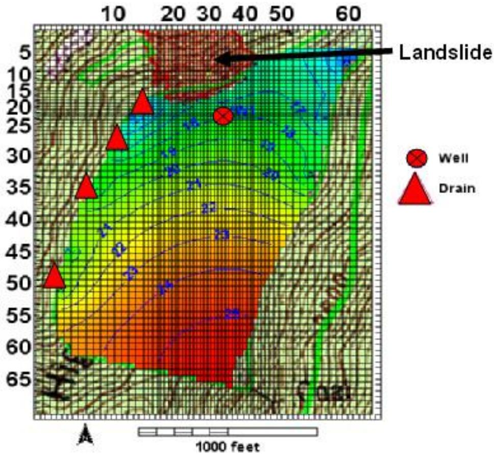
Figure 10. MODFLOW Grid Layout
