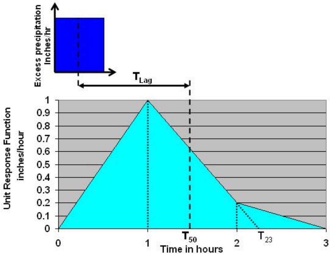
Figure 12. Ordinates of synthetic hydrograph.
