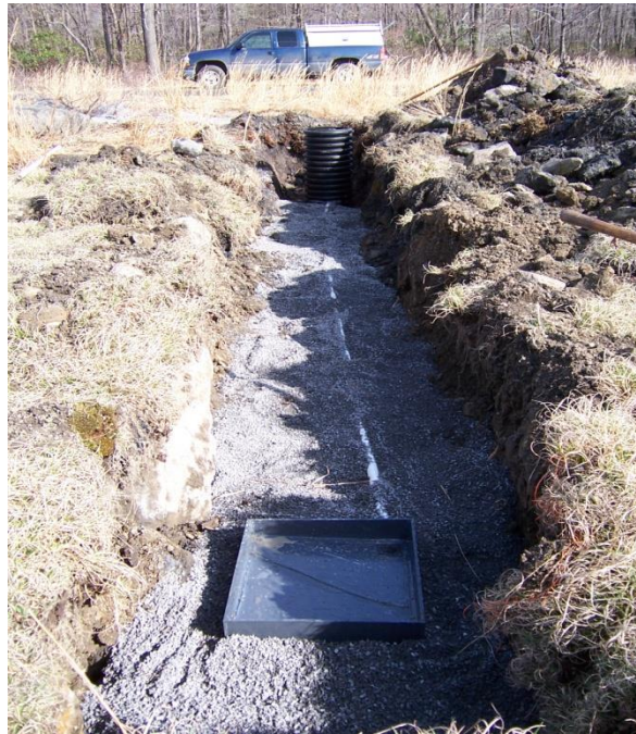
Figure 2. Pan lysimeter installation in the center of a plot. The leveled pan in the foreground drained to a carboy at the bottom of the PVC well in the background. The pan was then covered with the original soil removed from the trench.
