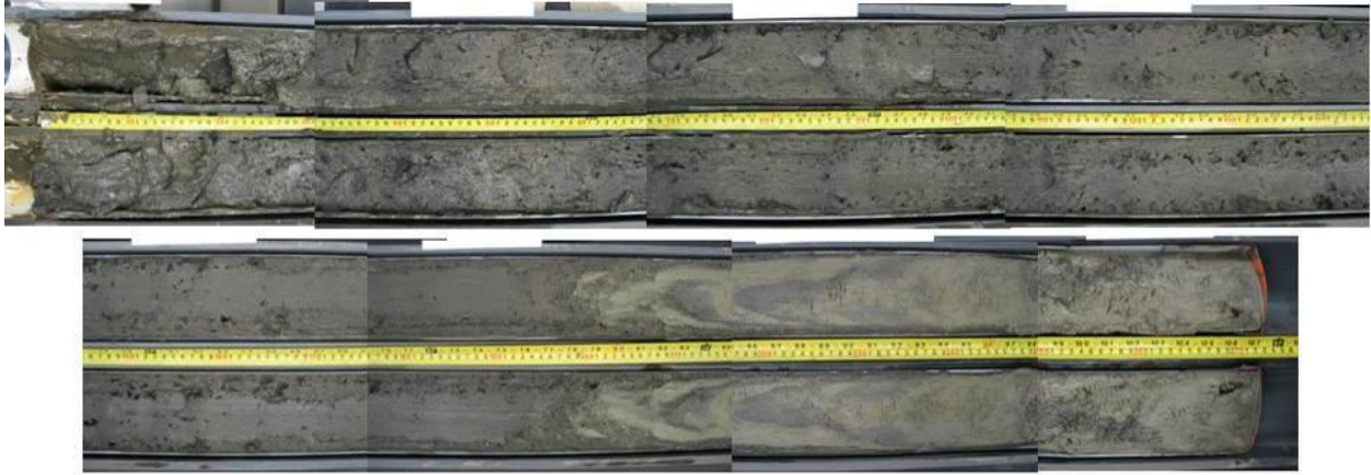
Figure 3. Mosaic of sediment core (SWS 357) collected with a vibracoring device. Top of core upper left, bottom of core lower right, length of core is 273 cm. Note dark color and fluid nature of upper core, and the low organic matter sediment that starts in the middle of the lower section at about 200 cm indicating pre-settlement deposition.
