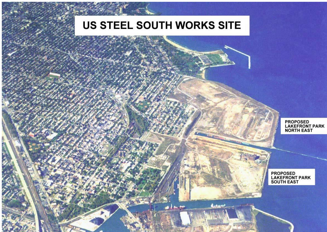
Figure 4. Aerial view of the US Steel (USX) South Works site. Note barge slip bisecting property where the sediment was offloaded from the barges to off-road dump trucks.
