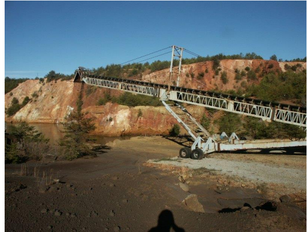
Figure 10A and 10B. Phase One Removal for Disposal in Isabella Collapse – Loading onto the Conveyor.
