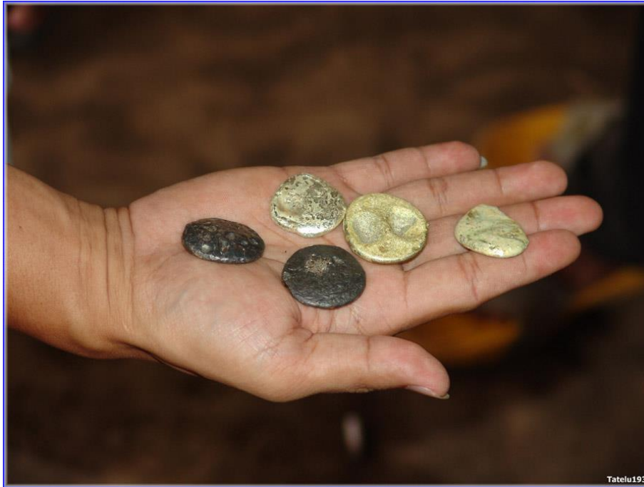
Figure 20. The yellow-gold buttons contain mostly Au, according to the Au buyers. The black buttons contain high Ag in addition to Au. The more valuable Au buttons were produced directly from Hg amalgamation. The Ag- Au buttons were produced by cyanidation. Because cyanidation recovers both Au and Ag more efficiently than amalgamation, it maximizes resource recovery. However, Au buttons command a higher price and thus may inhibit the switch from Hg amalgamation to cyanidation alone.
