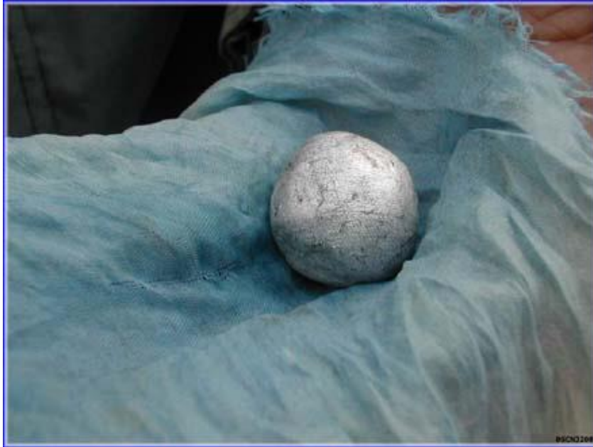
Figure 5. Gold-mercury amalgam after excess mercury and water has been squeezed through a dense cloth. This amalgam will be heated to drive off the mercury, leaving a button of Au.
