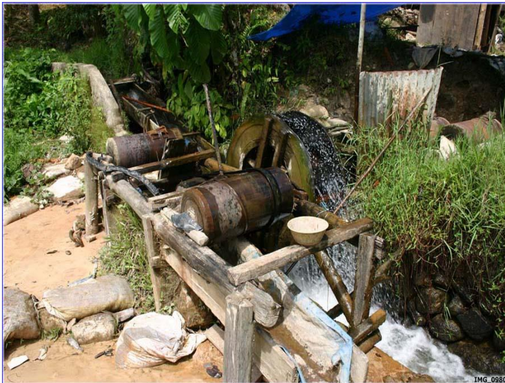
Figure 4. Water powered trommels, Pasaman, West Sumatra. A water wheel is used to turn two trommels in this set up.
