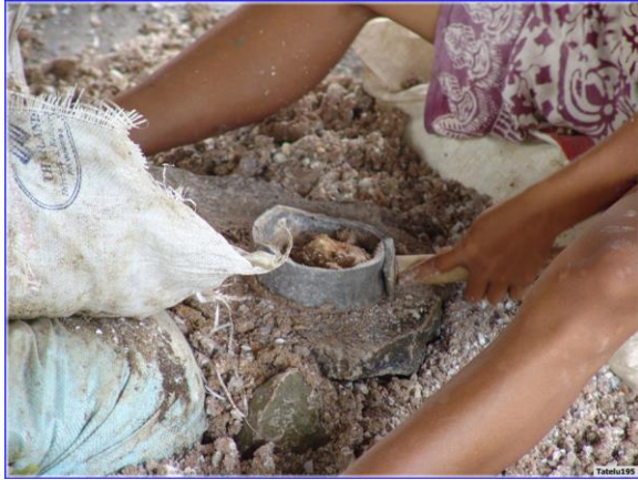
Figure 8. Ore is held inside a ring of conveyor belt material attached to a handle and crushed by hand with a hammer.
