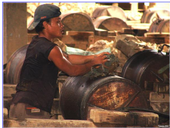
Figure 11. A worker loads ore for a second (or more) pass at crushing. If the crushed ore contains Hg, the workers' skin is exposed to it, especially through cuts or abrasions.
