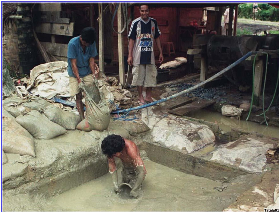
Figure 19. Recovering Hg-treated tails for Hg re-processing or cyanidation. Protective equipment is rarely available. Workers who are exposed to Hg contact in settings like these may limit their health or life span significantly through dermal contact alone.
