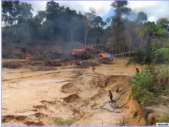
Figure 17. Gold is recovered from colluvium or paleo placers using hydraulic mining techniques. This technique releases massive amounts of sediment to streams and causes erosion and mass wasting.
