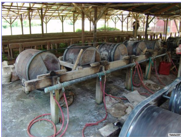
Figure 10. Trommel bank. Each drum, or trommel, holding about 20kg of ore is tumbled with river rocks for several hours. This autogenous grinding process is followed by further grinding with Hg to contact the Au with Hg to form an amalgam.
