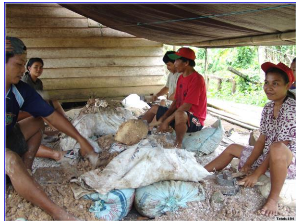
Figure 7. Community of workers using hammers to crush ore; Tatelu district.
