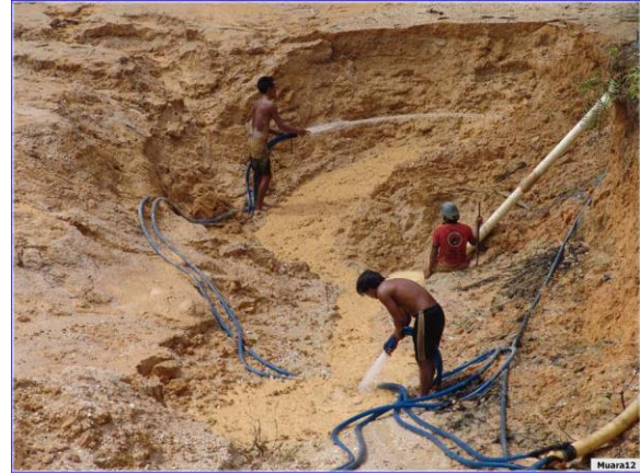
Figure 18. Hydraulic mining. A jet of water is sprayed at the loose sediment to expose Au bearing units. Valuable units will be run through sluice boxes to recover Au and heavy minerals.
