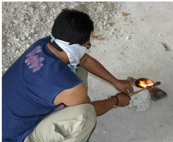
Figure 12. Amalgamated Au is heated with fluxes in an open clay or metal pot. The amalgam at this stage is unprotected, and Hg escapes to the open air.
