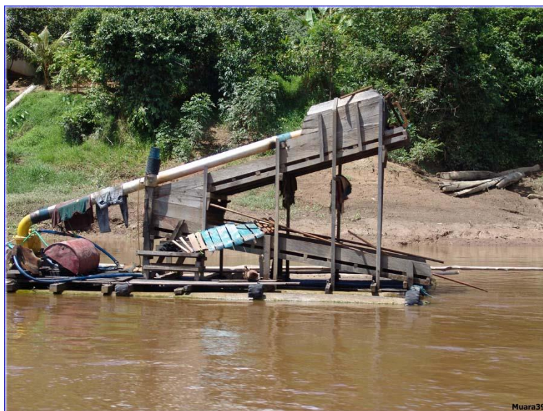
Figure 16. A suction dredge and sluice (tilted portions) recover free Au by gravity separation. Gold and other heavy minerals will be amalgamated and roasted to free the Hg. Barito River, Central Kalimantan.
