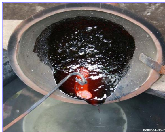
Figure 13. Gold button recovered after heating. Workers in this setting have the maximum contact with Hg vapors, and thus are most susceptible to Hg poisoning.
