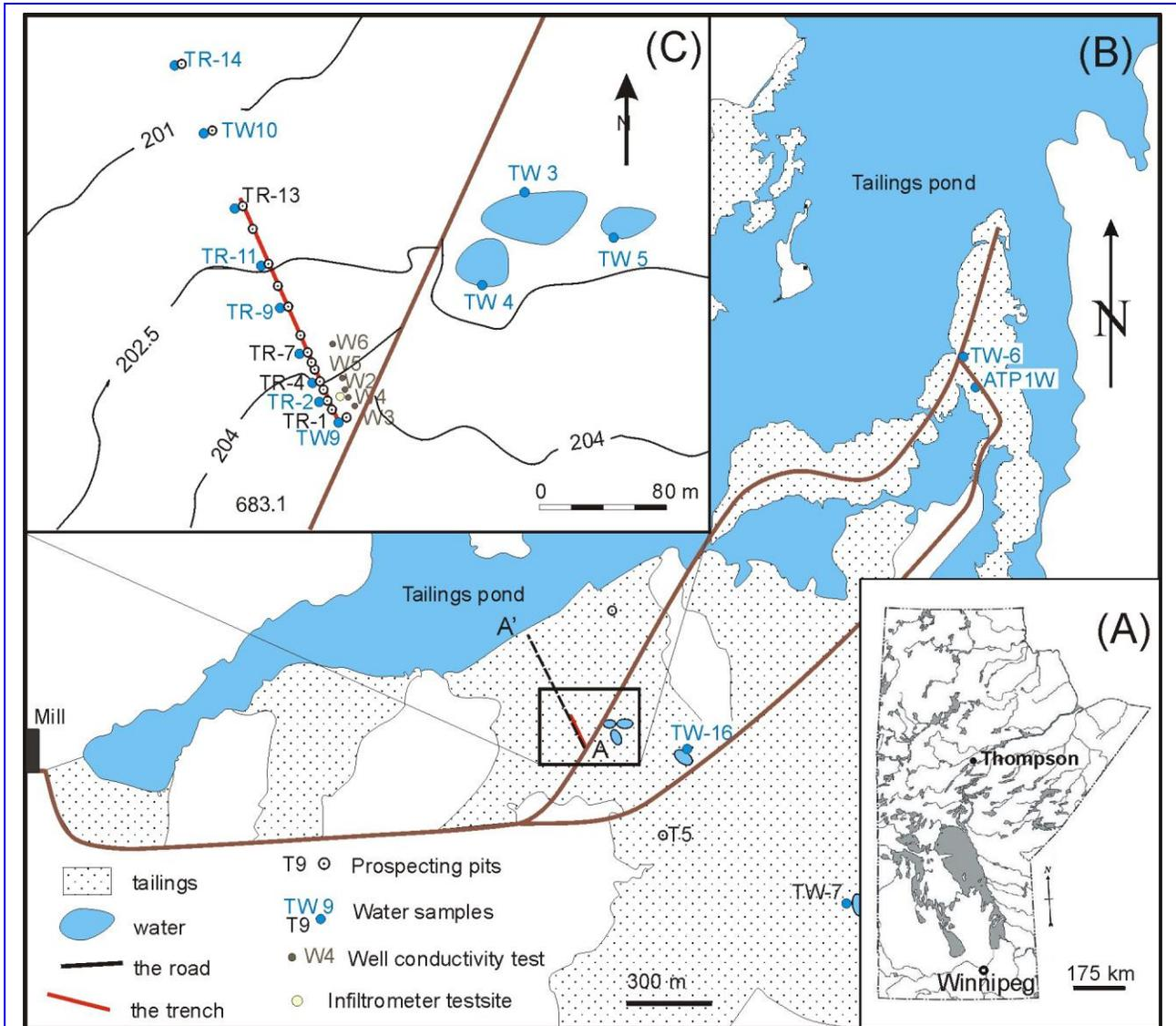
Figure 1. (a) A map showing the location of the INCO Ltd. Ni-Cu mine in Thompson, Manitoba, (b) a plan of the tailings showing trench and (c) the sampling points.
