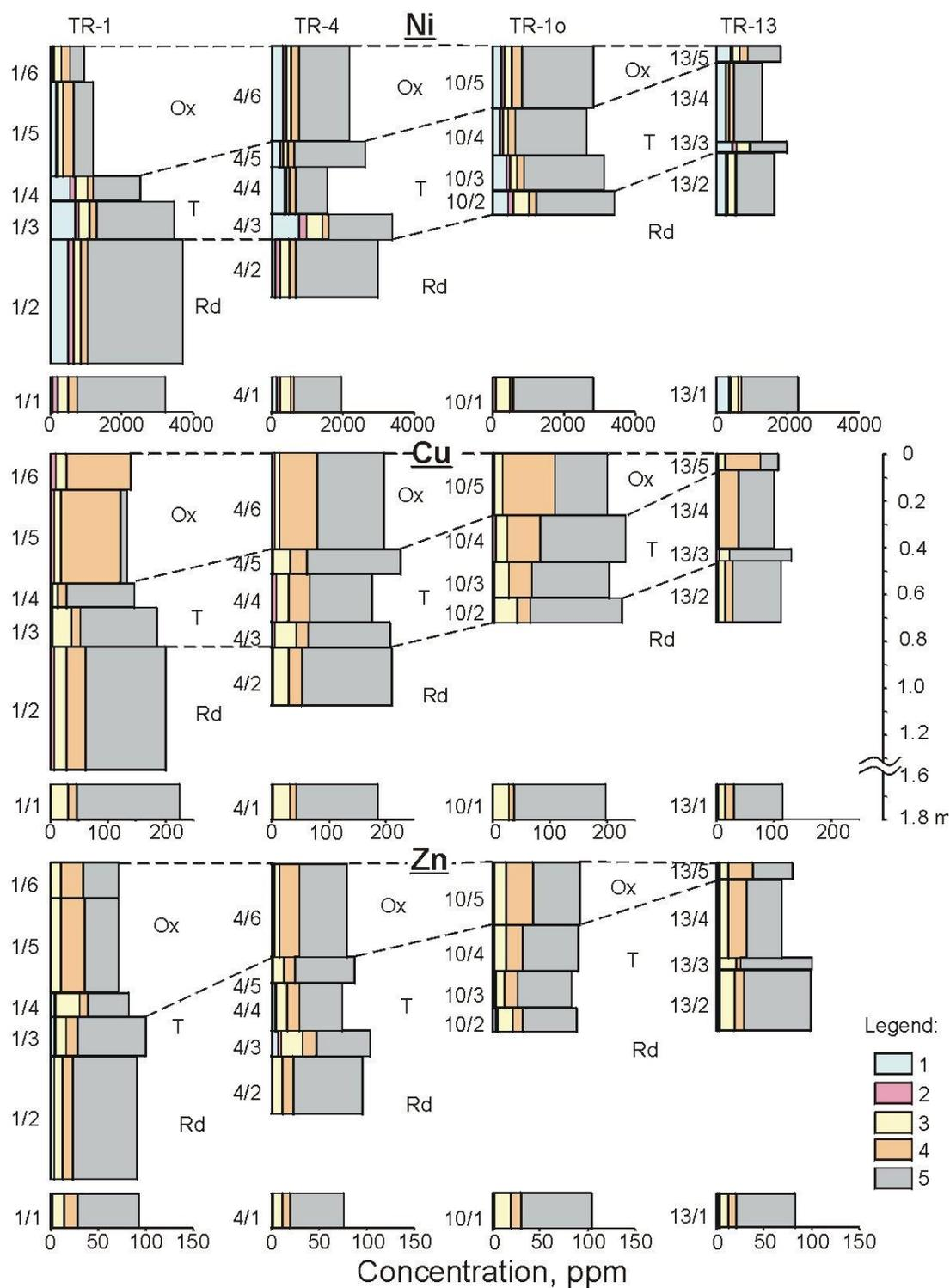
Figure 6. The distribution of Ni, Cu and Zn in vertical sections of the tailings. The fractions are (1) water-soluble fraction (2) exchangeable and carbonate, (3) bound to amorphous and poorly crystalline Fe-oxyhydroxides and oxyhydroxysulfates, (4) bound to crystalline Fe-oxyhydroxides and oxyhydroxysulfates, (5) residual.
