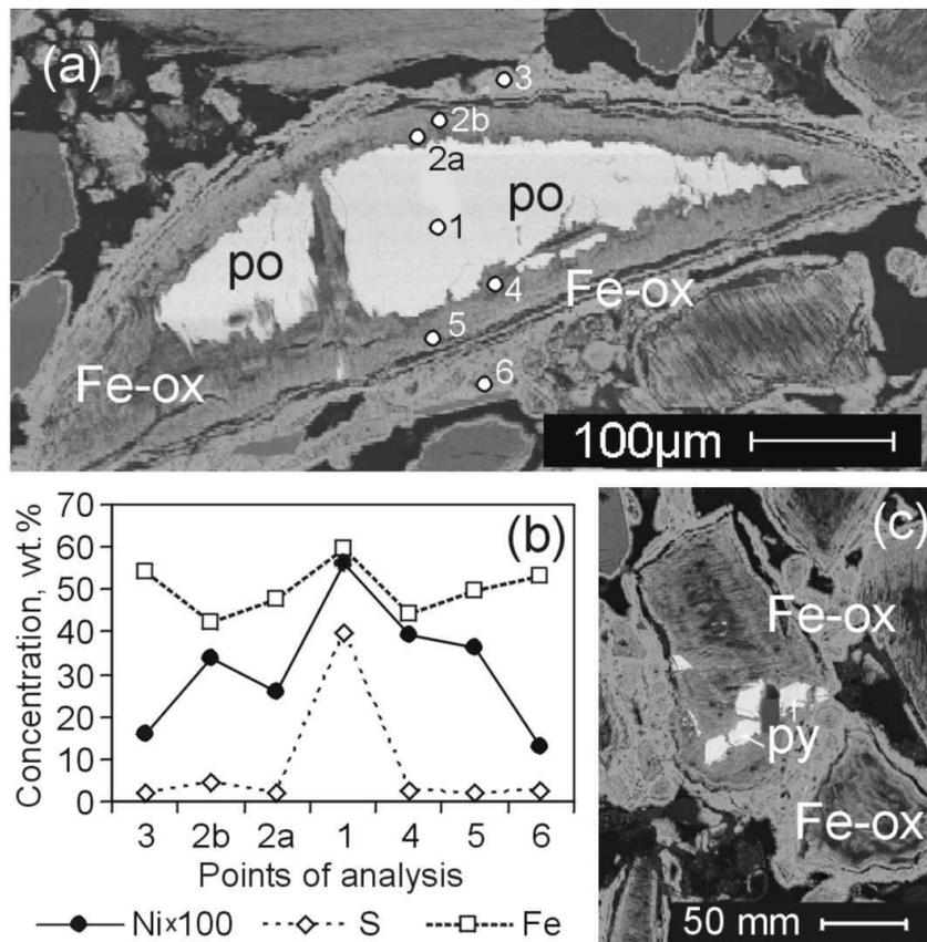
Figure 4. Scanning electron microscope images in electron backscattered mode and the results of EMP analyses showing: (a) pyrrhotite grain surrounded by Fe-oxyhydroxides with points of analyses through a rim-core-rim profile; (b) the concentration of Ni, S and Fe across the profile; (c) a grain of pyrrhotite almost completely replaced by Fe-oxyhydroxides containing inclusions of pyrite, sample 1/5.
