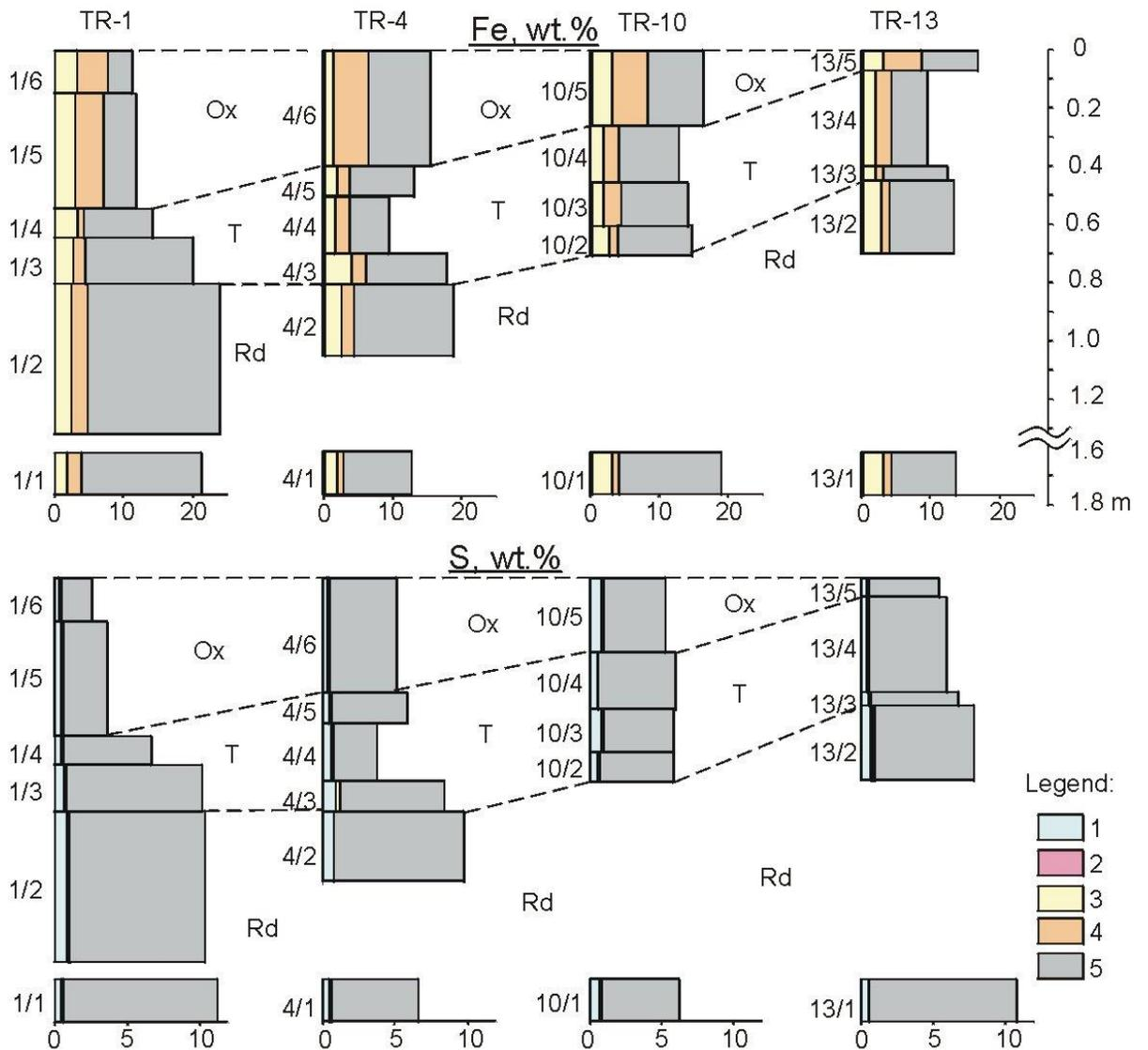
Figure 5. The speciation of Fe and S in the tailings solids from sequential extraction. The fractions are (1) water-soluble fraction (2) exchangeable and carbonate, (3) bound to amorphous and poorly crystalline Fe-oxyhydroxides and oxyhydroxysulfates, (4) bound to crystalline Fe-oxyhydroxides and oxyhydroxysulfates, (5) residual.
