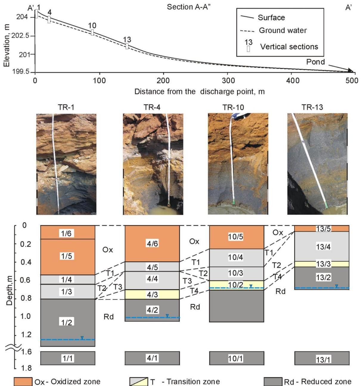
Figure 2. The position, and photographs of the vertical sections and the location of samples in these sections. Zones are correlated between different sections of the trench. Zone names: Ox – Oxidized zone, T1-T4–Transition zone, Rd – Reduced zone. The dashed line with triangles shows the level of the water table. The scale bar of the photographs is 0.5m.
