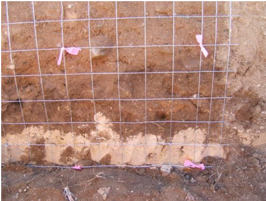
Figure 3. Tonguing of tailing in the basal contact zone of a soil cover overlying tailing. Wire mesh grid spacing is 10 cm.
