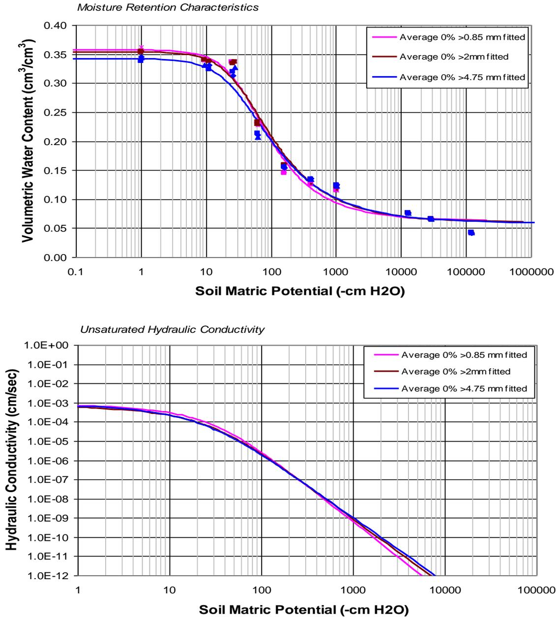
**Figure 5.** Mualem-van Genuchten predicted MRC curves and hydraulic conductivity-matric potential functions for fine-earth samples.
