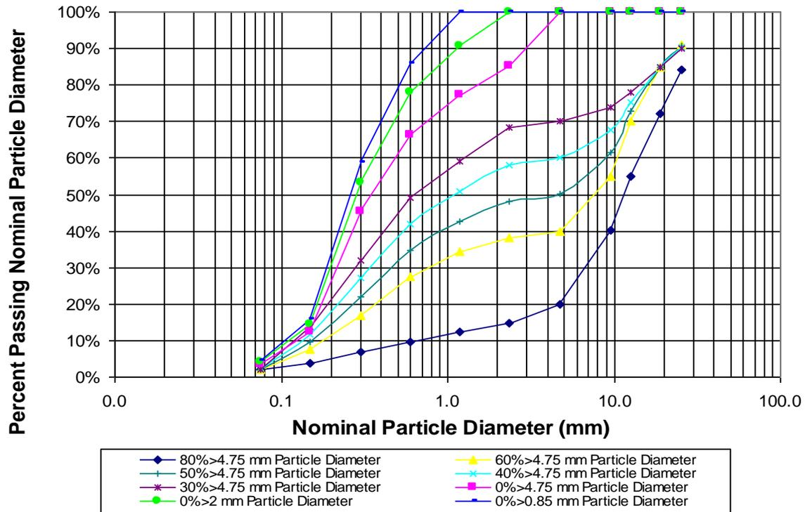
Figure 3. Particle size distribution of fabricated soils.
