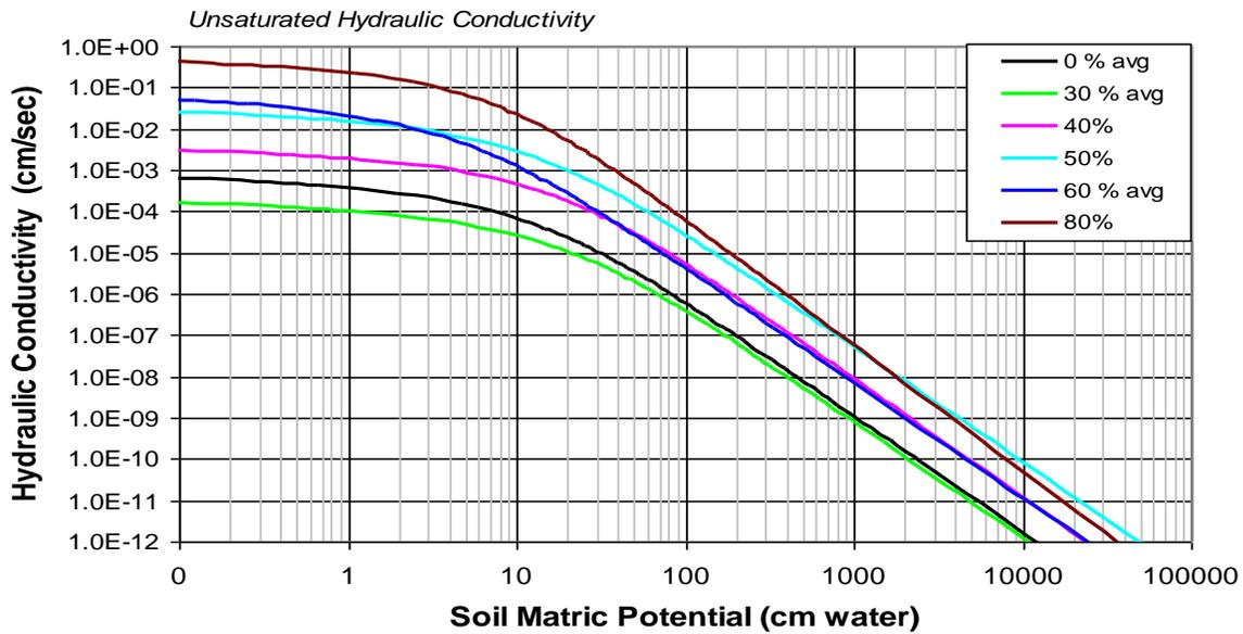
**Figure 6.** Mualem-Van Genuchten predicted MRC curves and hydraulic conductivity-matric potential functions for all samples.
