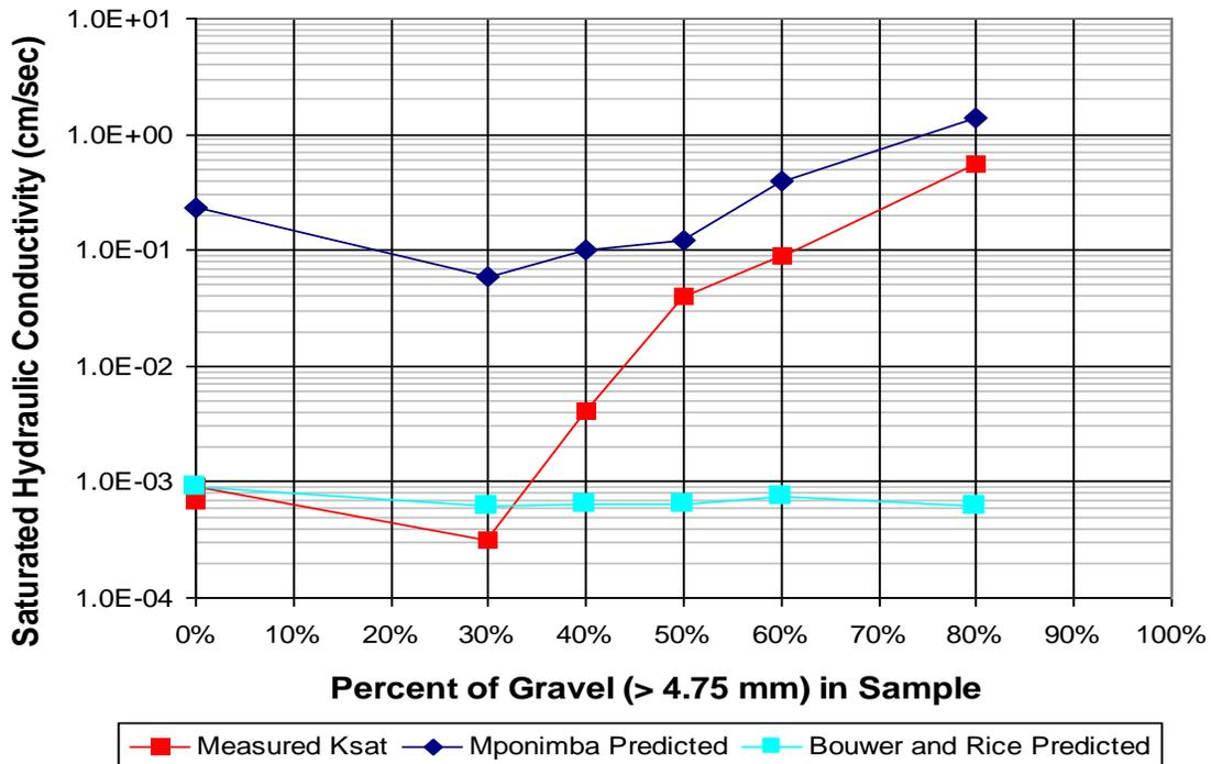
Figure 4. Measured saturated hydraulic conductivity vs. percent of gravel in sample.
