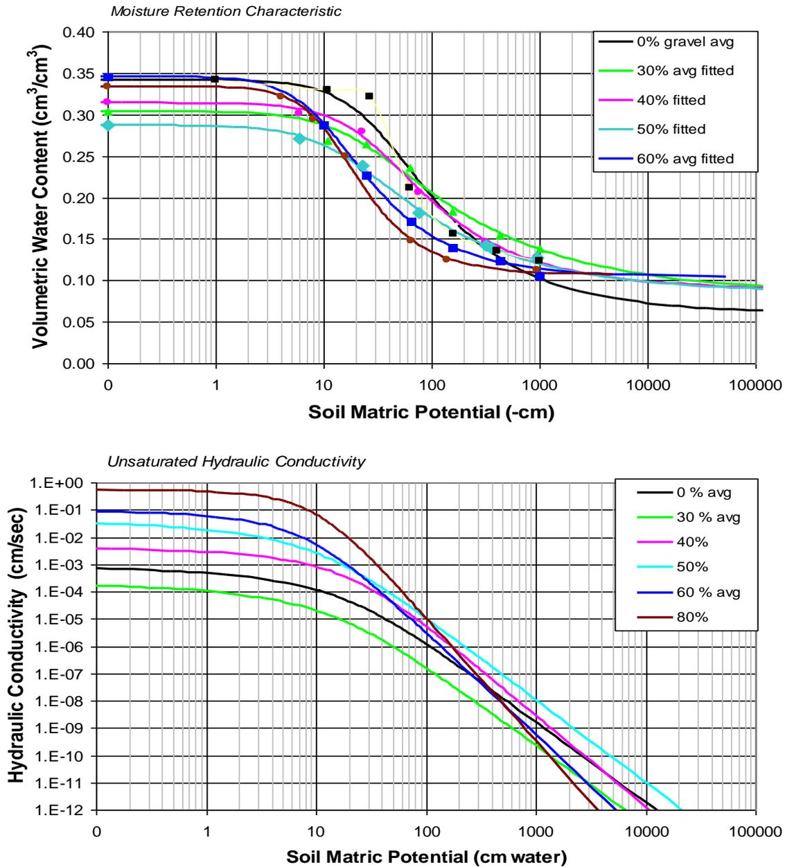
Figure 9. Results of fixing the residual water content values between 6 to 10% for the Mualem-Van Genuchten predicted MRC curves and hydraulic conductivity-matric potential functions.
