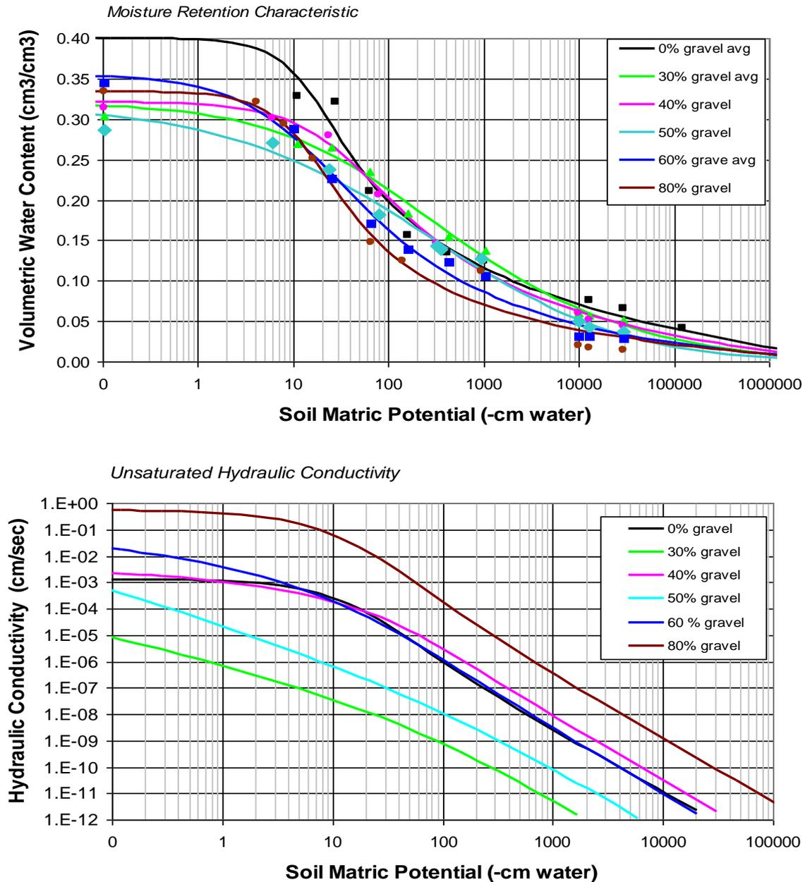
Figure 7. Fredlund and Xing predicted MRC curves and hydraulic conductivity-matric potential functions for all samples.
