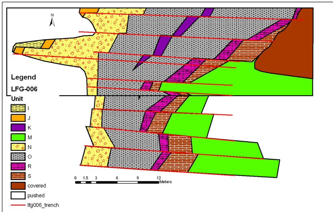
Figure 7. Geologic map of trench LFG-006, stable portion of GHN. Units are described below in Table 2. Offsets show bench wall locations and are not faults. Red lines indicate the edge of each bench. The units closest to the base of the rock pile (east) are older than the younger, overlying units towards the outer edge of the rock pile (west).
