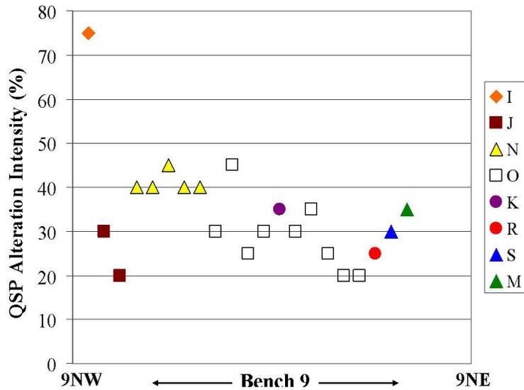
Figure 11. Plot of QSP hydrothermal alteration intensity (defined by the percentage of hydrothermal alteration minerals that have replaced primary minerals) across bench 9, trench LFG-006. Refer to Figure 9 for geologic section.
