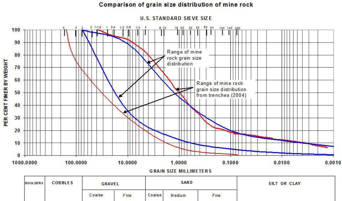
Figure 8. Grain size analyses of selected samples from GHN compared to data contained in earlier Molycorp reports. The red lines are from data in URS Corporation (2000) and the blue lines are from data obtained in this study from GHN.
