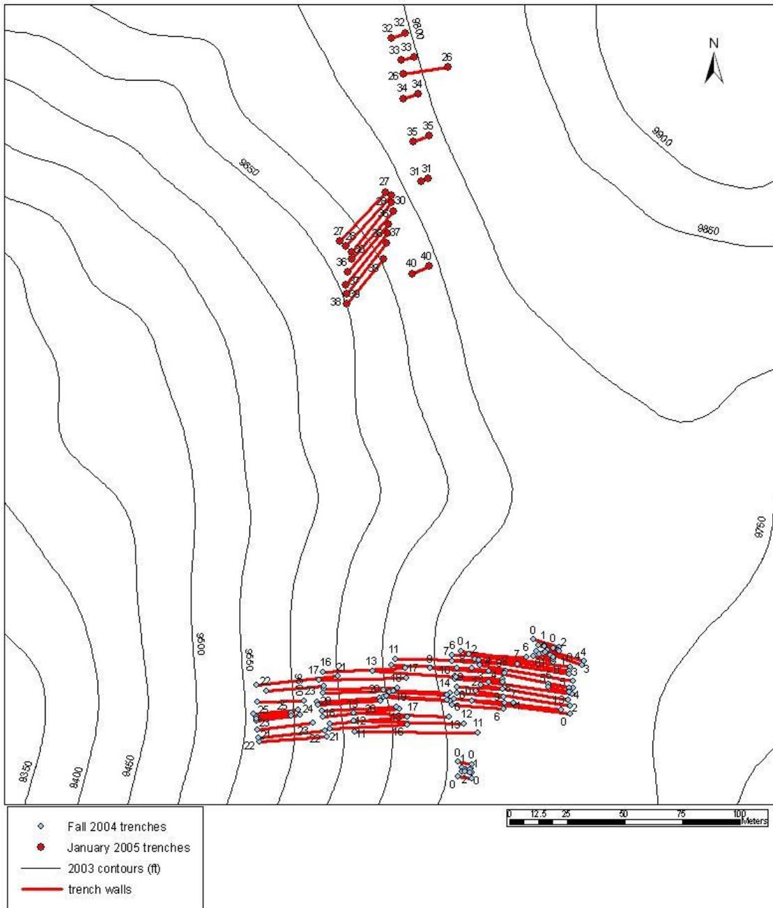
Figure 6. Map showing GHN trench locations. Red lines show trench walls. Circles show surveyed trench corner points. Black lines show elevation contours. Numbers refer to bench numbers.
