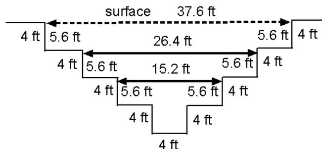
Figure 4. Sketch of a typical trench for the GHN rock pile.
