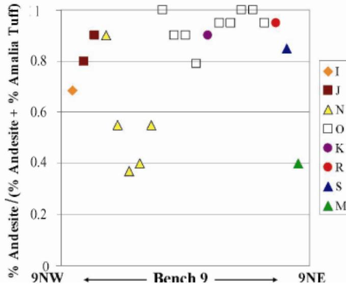
Figure 10. Plot of rock fragments lithology (normalized to andesite + Amalia Tuff) across bench 9, trench LFG-006. Outer oxidized, margin of rock pile is on the left (refer to Figure 9 for geologic section).
