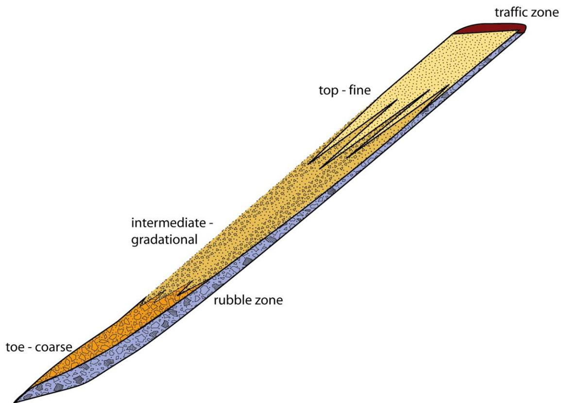
Figure 3. Conceptual model of the Questa rock piles (from field studies at GHN and from Nichols, 1987). See text below and McLemore et al. (2005) for explanation of zones.
