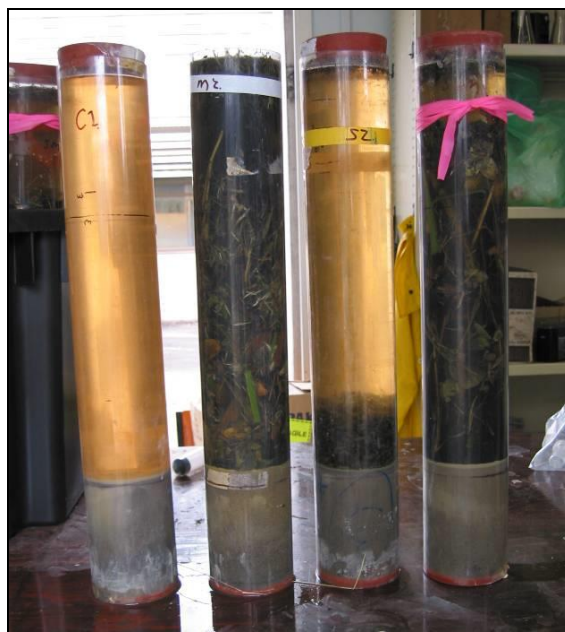
Figure 5. Microcosm cores on day 0. Treatment allocations from left to right are control, green waste, sewage and green waste and sewage.
