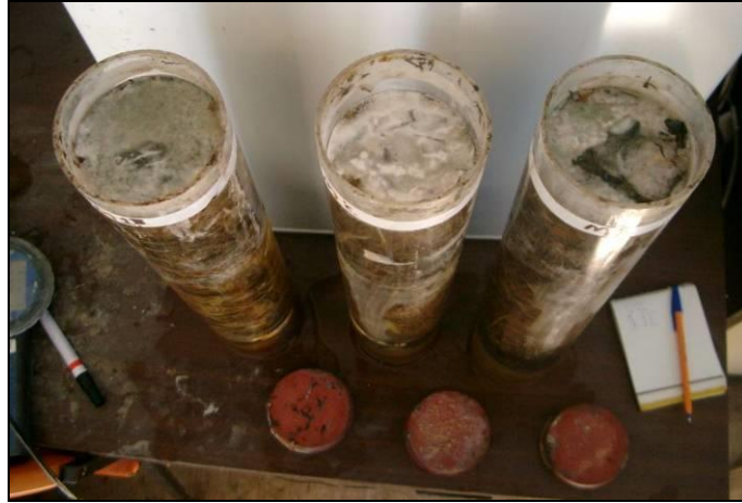
Figure 6. Mould growing on the surface of green waste-only cores at day 72.
