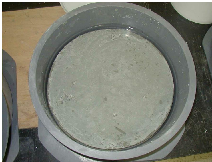
Figure 1. Top view of cemented paste in kinetic test cell.
