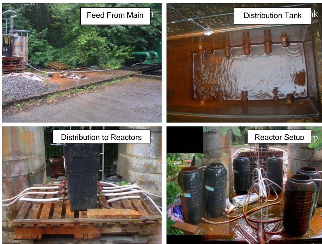
Figure 2. Photographs of the pilot scale reactors, including the influent feed and distribution system.
