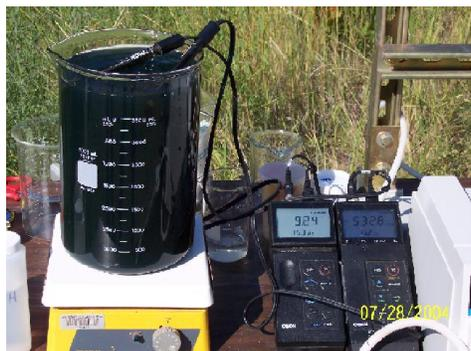
Figure 3. Susie/Valley Forge Mine water treated with NaOH.
