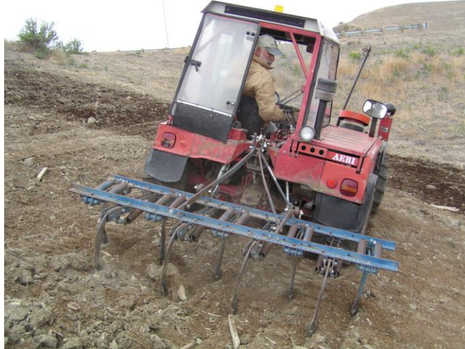
Figure 17. Ford spring-shanked tiller on Plot 20 (Rocky Mountain compost in foreground, Earth Systems material in background).
