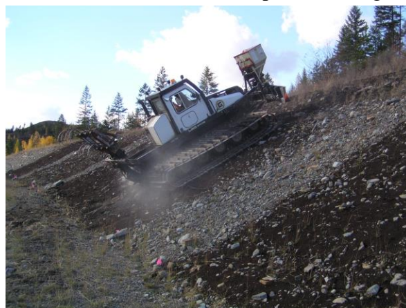
Figure 13. Modified LMC 3700C initiating tillage on plot 8, Loon Lake site.
