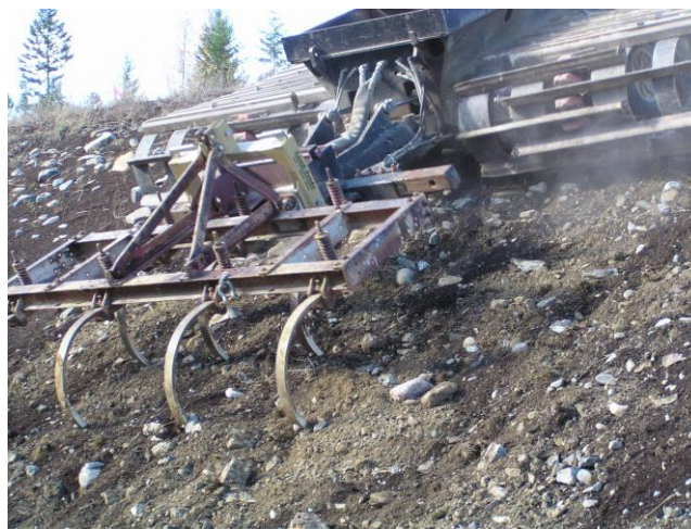
Figure 14. Graham Hoeme 2.4 m (8 ft) spring shanked chisel plow at Loon Lake.
