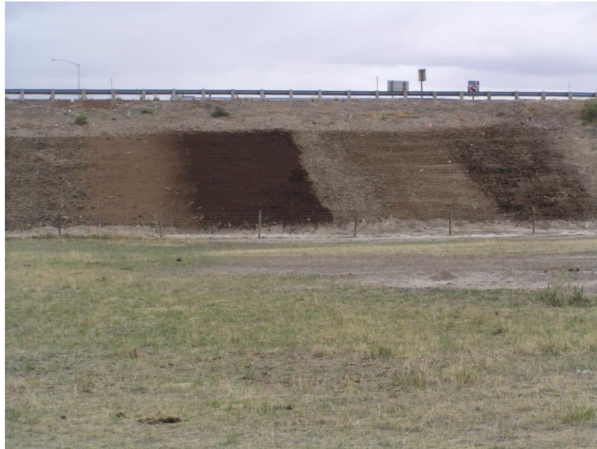
Figure 9. Plots 19 (compost blanket) and 20 (incorporated compost), I-94 off-ramp area, showing Rocky Mountain compost on the left (light-colored) and Earth Systems compost on the right (dark-colored)
