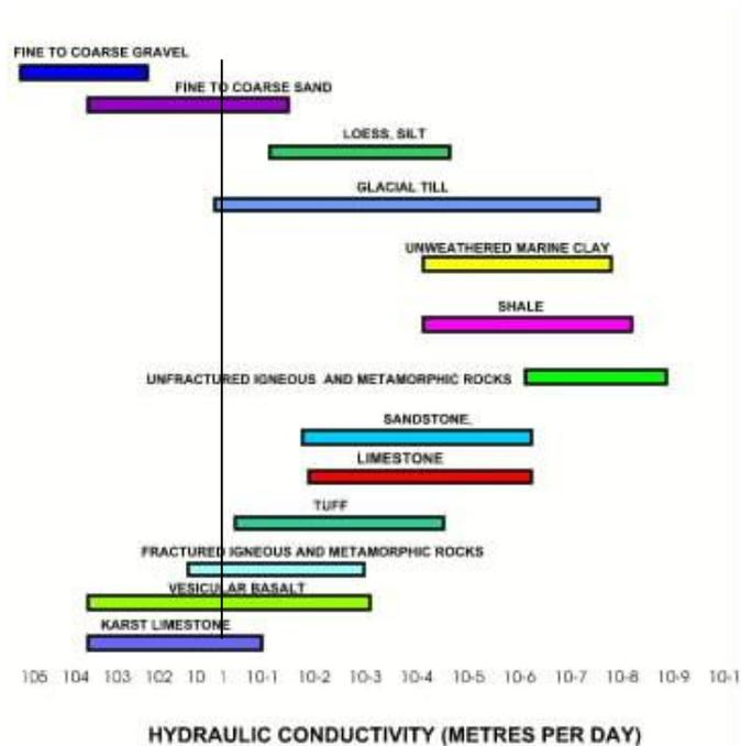
Figure 5 Diagram of typical hydraulic conductivities with the average conductivity for this experiment shown with the vertical line. From [http://wvlc.uwaterloo.ca/biology447/modules/module7/images/7a\\_s1g5.jpg](http://wvlc.uwaterloo.ca/biology447/modules/module7/images/7a_s1g5.jpg)
