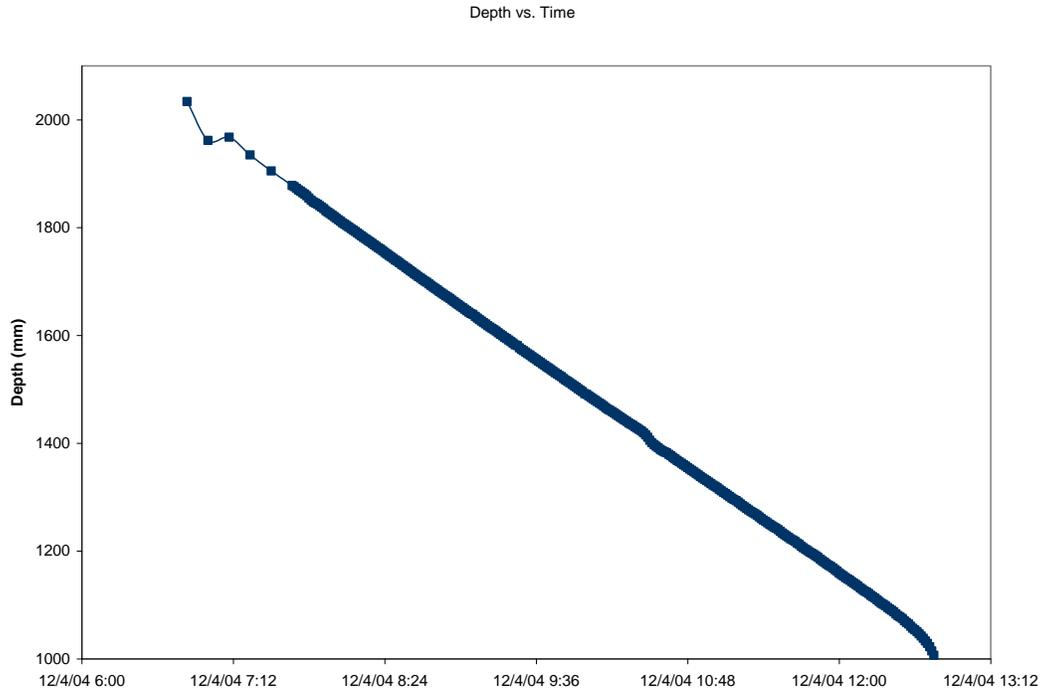
Figure 3 Depth of standing water vs. time for field scale falling head test of 12/4/04.
