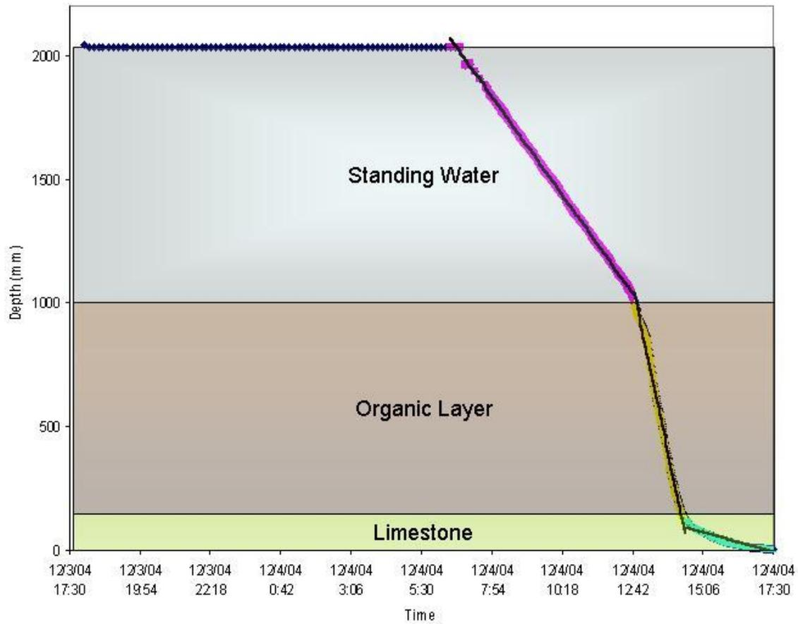
Figure 2. Field data collected from falling head test conducted 12/4/04. Bold line indicates depth of water above the logger.
