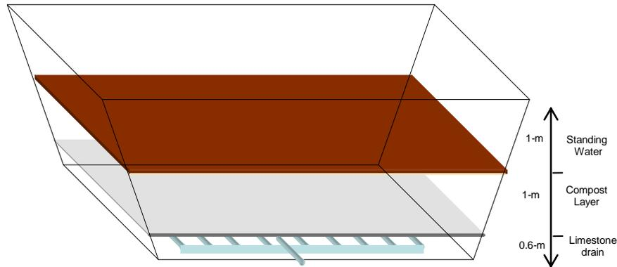
Figure 1. Conceptual design schematic of Cell 4 vertical flow system unit at the Red Oak passive treatment system.
