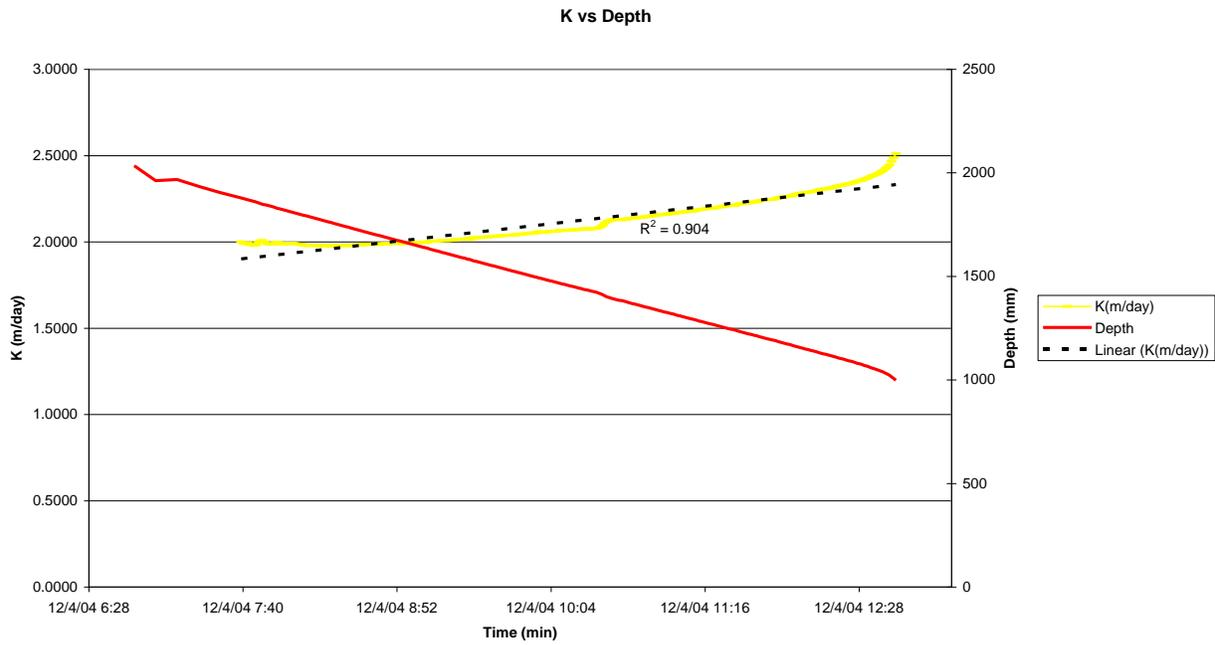
Figure 4. Hydraulic conductivity vs. depth for standing water portion of Cell 4. Trend line shows  $R^2$  value.
